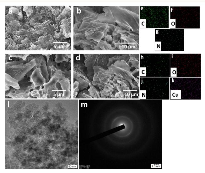
Fig. 3 SEM micrographs of POPs (a and b) and POP-Cu(II) sorbent (c and d) at different magnifications and their respective elemental analysis (e-k); TEM micrograph of POPs (I) and the corresponding SAED pattern, illustrating the amorphous morphology of POPs (m).
