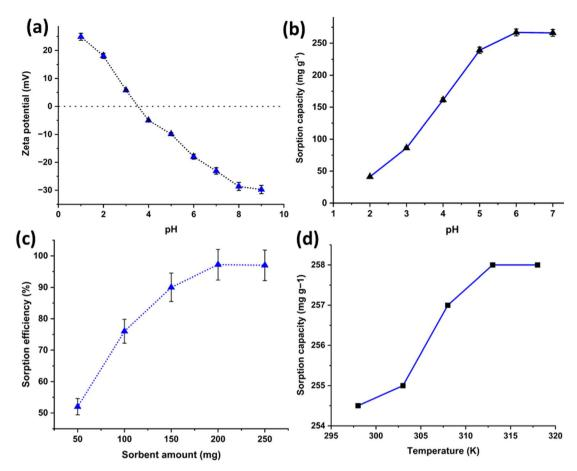
Fig. 4 (a) Zeta potential of the measurement of POPs; (b) effect of the solution pH on Cu(II) adsorption, (sample volume, 100 mL; concentration, 500  $\mu$ g mL<sup>-1</sup>; sorbent amount, 200 mg; flow rate, 5 mL min<sup>-1</sup>); (c) effect of the sorbent amount on Cu(II) adsorption, (sample volume, 100 mL; concentration, 10  $\mu$ g mL<sup>-1</sup>; sample, pH 6; flow rate, 5 mL min<sup>-1</sup>); (d) effect of temperature on the adsorption of metal ions.
