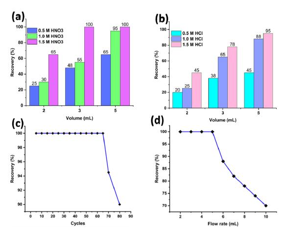
Fig. 5 (a and b) Effect of various eluting agents on the recovery of the sorbed amount of Cu(II), (sample volume, 100 mL; concentration, 50 μg  $mL^{-1}$ ; sample, pH 5; eluent flow, 2 mL min<sup>-1</sup>); (c) reusability of the POP sorbent for multiple adsorption–desorption cycles; (d) effect of the flow rate on the sorption of metal ions.
