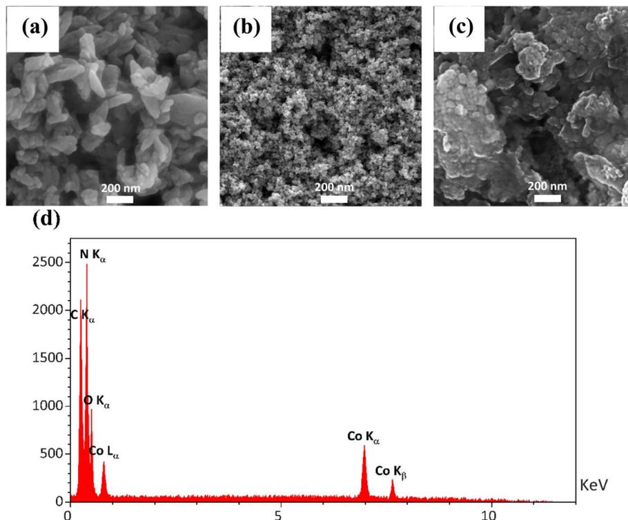
Fig. 3 FESEM image of (a) g-C<sub>3</sub>N<sub>4</sub> nanoplates, (b) LiCoO<sub>2</sub> nanoparticles, and (c) GL3 hybrid materials. (d) EDX spectra of GL3 sample.
