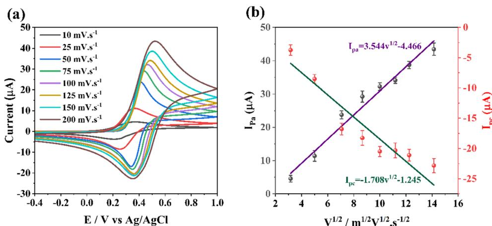
Fig. 8 (a) CV curves of g-C<sub>3</sub>N<sub>4</sub>@LiCoO<sub>2</sub>/GCE in PBS (pH 7) containing 10 nM malathion at various scan rates. (b) The curves of anodic and cathodic peak currents regarding the square of scan rate.
