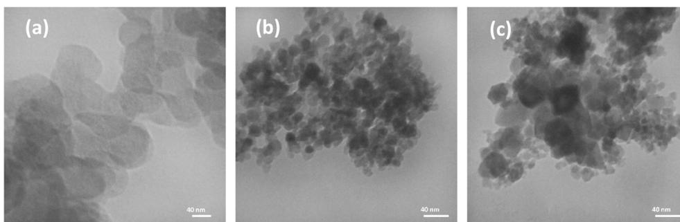
Fig. 4 TEM image of (a) g-C<sub>3</sub>N<sub>4</sub> nanoplates, (b) LiCoO<sub>2</sub> nanoparticles, and (c) GL3 hybrid materials.
