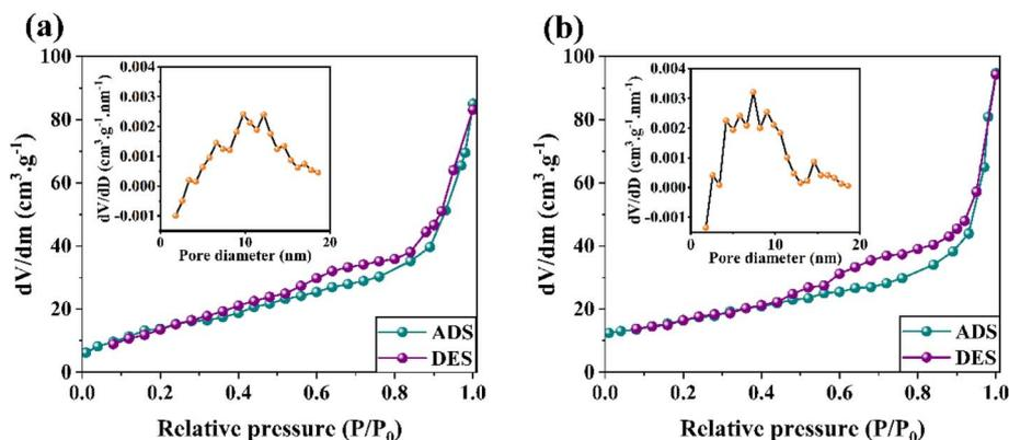
Fig. 6  $\text{N}_2$  adsorption–desorption response and BJH pore size distributions of (a)  $g\text{-C}_3\text{N}_4$  and (b) GL3 samples.
