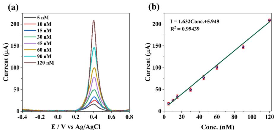
Fig. 9 (a) DPV plots for different concentrations (5–120 nM) of malathion based on the g-C<sub>3</sub>N<sub>4</sub>@LiCoO<sub>2</sub>/GCE electrode at pH 7 (0.1 M PBS solution). (b) The calibration curve of DPSV current at the g-C<sub>3</sub>N<sub>4</sub>@LiCoO<sub>2</sub>/GCE electrode versus malathion concentration.
