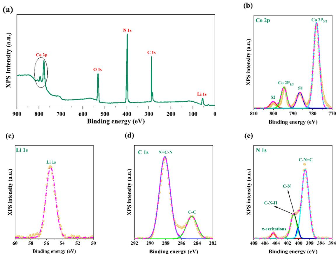
Fig. 5 (a) XPS spectra of GL3 sample. High-resolution XPS for (b) Co 2p, (c) Li 1s, (d) C 1s, and (e) N 1s elements.
