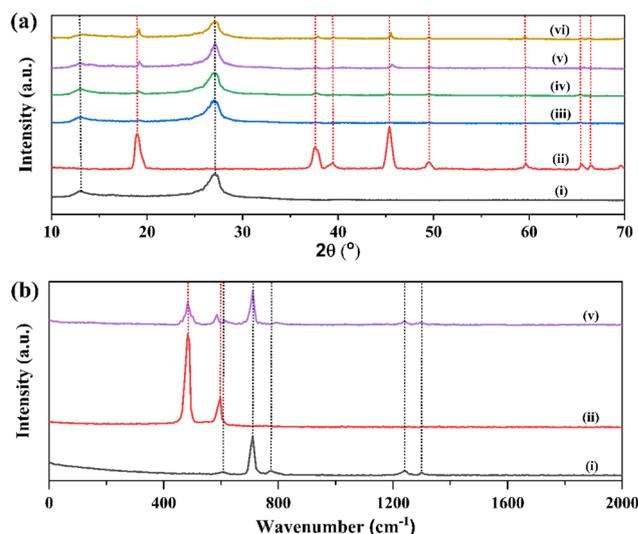
Fig. 2 (a) XRD pattern and (b) Raman spectra of different samples. (i)  $g\text{-C}_3\text{N}_4$ , (ii)  $\text{LiCoO}_2$ , (iii) GL1, (iv) GL2, (v) GL3, and (vi) GL3.
