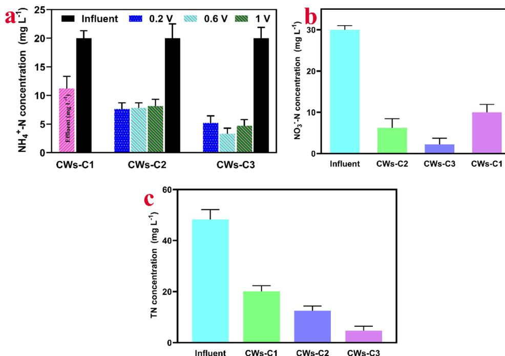
Fig. 3 (a) The performance of CWs in the  $\text{NH}_4^+$ -N removal at different applied potential; (b) and (c) the  $\text{NO}_3^-$ -N and TN removal at constant applied potential of 0.6 V (*versus* Ag/AgCl). (note: the operation period for all parameters were 45 days with HRT of 2 days, every 5 days parameters were measured).
