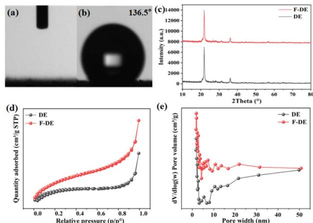
Fig. 1 CA photos of DE (a) and F-DE (b), XRD spectra (c), N<sub>2</sub> adsorption/desorption isotherms (d) and pore width distribution curves (e).
