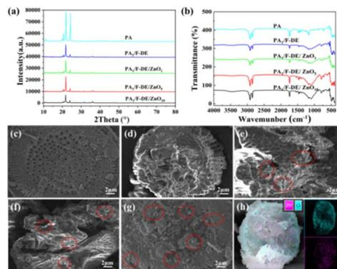
Fig. 3 XRD (a) and FTIR (b) of PA and PA<sub>1</sub>/F-DE/ZnO composite PCMs, SEM images of F-DE (c), PA<sub>1</sub>/F-DE (d), PA<sub>1</sub>/F-DE/ZnO<sub>1</sub> (e), PA<sub>1</sub>/F-DE/ZnO<sub>5</sub> (f), PA<sub>1</sub>/F-DE/ZnO<sub>10</sub> (g), and EDS of PA<sub>1</sub>/F-DE/ZnO<sub>10</sub> (h).
