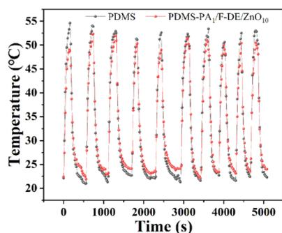
Fig. 8 Temperature changes of PDMS-PA<sub>1</sub>/F-DE/ZnO<sub>10</sub> for 10 cycles heating and cooling.
