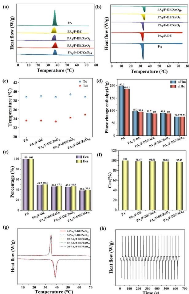
Fig. 4 DSC curves of PA, PA<sub>1</sub>/F-DE and PA<sub>1</sub>/F-DE/ZnO during endothermic (a) and exothermic (b) processes, and their melting ( $T_m$ ) and crystallization temperature ( $T_c$ ) (c), phase change enthalpy (d), encapsulation rate ( $E_{en}$ ), encapsulation efficiency  $E_{es}$  (e) and thermal storage efficiency  $C_{es}$  (f), and DSC curves of PA<sub>1</sub>/F-DE/ZnO<sub>10</sub> after experiencing 20 heating-cooling cycles (g and h).
