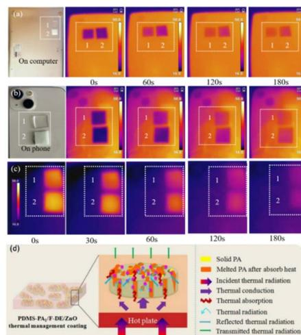
Fig. 9 Infrared thermal images of PDMS (1) and PDMS-PA<sub>1</sub>/F-DE/ZnO<sub>10</sub> (2) films placed on the back of a computer (a), a phone (b) and on a cold phone (c), the thermal management mechanism diagram of PDMS-PA<sub>1</sub>/F-DE/ZnO coating (d).
