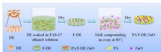
Fig. 2 Schematic illustration of the preparation for PA/F-DE/ZnO composite PCMs.
