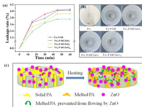
Fig. 6 The leakage rate (a), the photos of diffusion-permeation ring on the filter paper for 60 min (b) and the preventing leakage mechanism (c) of PA<sub>1</sub>/F-DE/ZnO composite PCMs.
