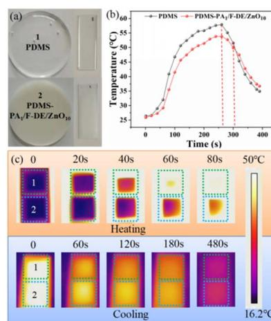
Fig. 7 Photographs of PDMS and PDMS-PA<sub>1</sub>/F-DE/ZnO<sub>10</sub> films and coatings on glass substrates (a), the temperature changes of film surface during heating and cooling with time (b) and thermal infrared images (c).
