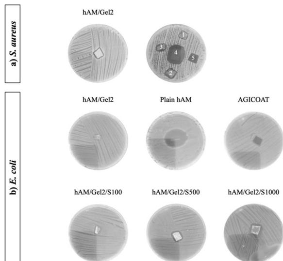
Fig. 10 Disc diffusion antibacterial test of plain hAM, hAM/Gel2, hAM/Gel2/S and AGICOAT scaffolds against (a) *S. aureus* and (b) *E. coli*. The numbers 1, 2, 3, 4 and 5 in section (a) correspond to hAM/Gel2/S100, hAM/Gel2/S500, hAM/Gel2/S1000, plain hAM and AGICOAT, respectively.
