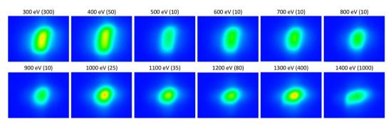
Fig. 5 Variation of the beam shape with the photon energy of the synchrotron radiations over 300-1400 eV. Numbers in parentheses are exposure times in the units of ms. The sensing area of the CMOS camera was  $4.97 \text{ mm} \times 3.73 \text{ mm}$ .
