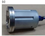
Fig. 4 (a) Bright-field image of an FOP without FND coating. Individual fibers of 6 μm in diameter can be readily seen for the FOP. (b) Exploded view of a fiber-coupled DEUVI system. (c) A prototype of fiber-coupled DEUVI.
