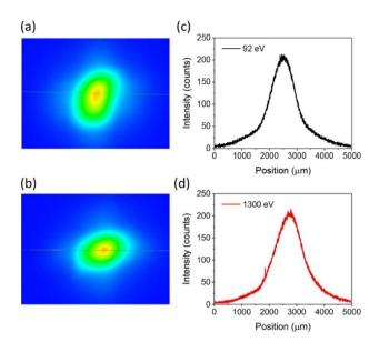
Fig. 7 (a and b) Images and (c and d) intensity profiles of synchrotron radiations at 13.5 nm (a and c) and 0.95 nm (b and d), obtained with a fiber-coupled DEUVI system. The beam flux was 7.7  $\times$   $10^{11}$  photons per s (and 4.5  $\times$   $10^{10}$  photons per s), and the exposure time used to acquire the image in (a) (and b) was 0.1 s (and 0.4 s) with a gain of 1 dB. The pixel size of the imaging sensor on the CMOS camera was 3.45  $\mu m$ .
