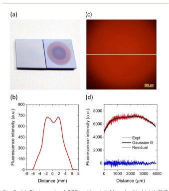
Fig. 3 (a) Photograph of FOPs without (left) and with (right) FND coatings prepared by electrospray deposition. Dimensions of the FOPs were  $14 \times 14 \text{ mm}^2$ . (b) Fluorescence intensity line profile across the center of an FND film on an FOP. (c and d) Wide-field fluorescence image (c) and fluorescence intensity line profile (d) of an FND film on an FOP. The white line in (c) denotes the data points in (d), which were fitted with two Gaussian functions (black)
