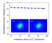
Fig. 6 Photostability tests of an FND scintillator with 13.5 nm radiation from the BL08B beamline. The beam flux used was  $7.7 \times 10^{11}$  photons per s with a beam spot area of  $\sim 0.46$  mm<sup>2</sup>. The measured fluorescence intensities were normalized by the photocurrents of a calibrated photodiode. (Inset) Images of the beam at the beginning (left) and end (right) of the measurements, showing a negligible change in beam profile after continuous operation for 6 h.
