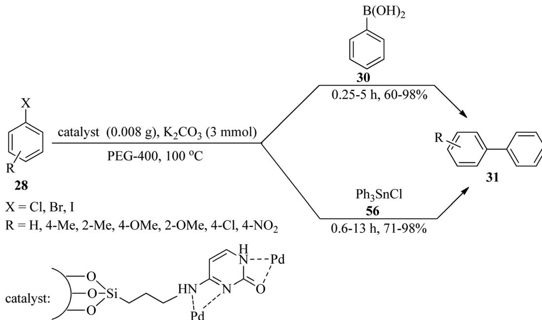
Scheme 34 Biphenyl synthetic routes in the presence of HMS-CPTMS-Cy-Pd.
