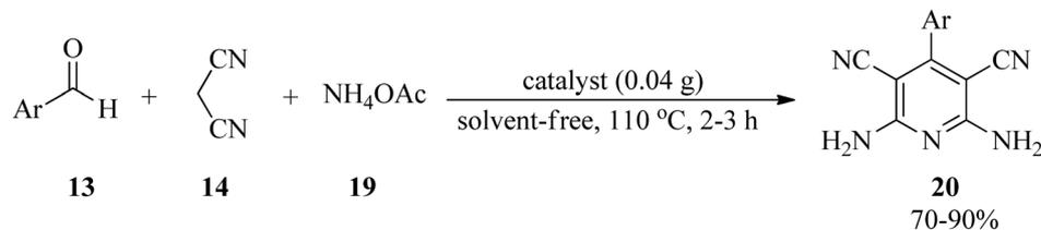
Ar = Ph, 4-ClPh, 2-ClPh, 4-OHPh, 3-NO<sub>2</sub>Ph, 2-NO<sub>2</sub>Ph, 4-CHOPh, 3-OMePh, 5-OMe-6-OHPh, 3-OMe-4-OHPh, 2-furanyl
