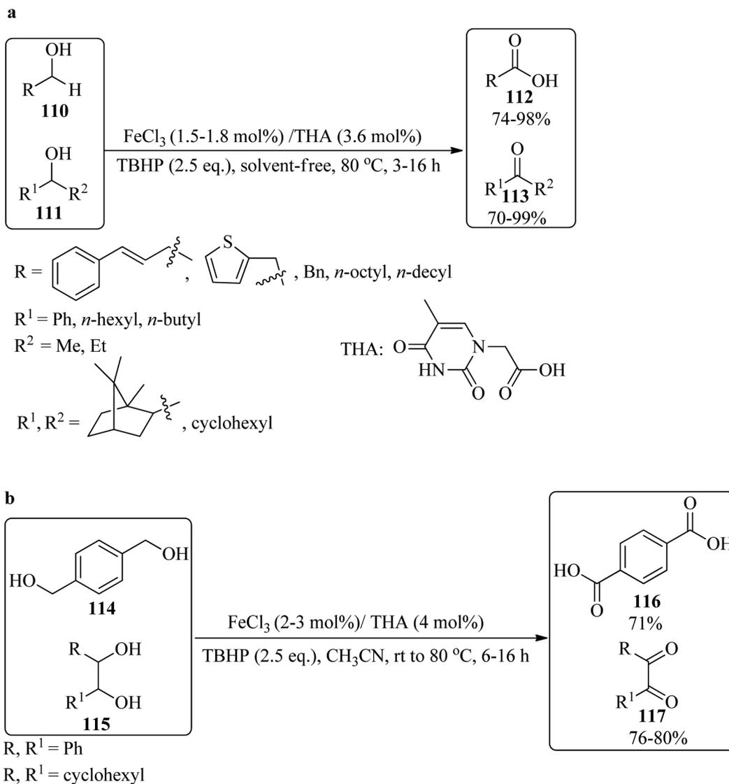
Scheme 36 Oxidation of (a) primary and secondary alcohols, and (b) diols.
