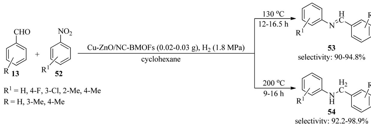
Scheme 16 Synthesis of imines and secondary amines.
