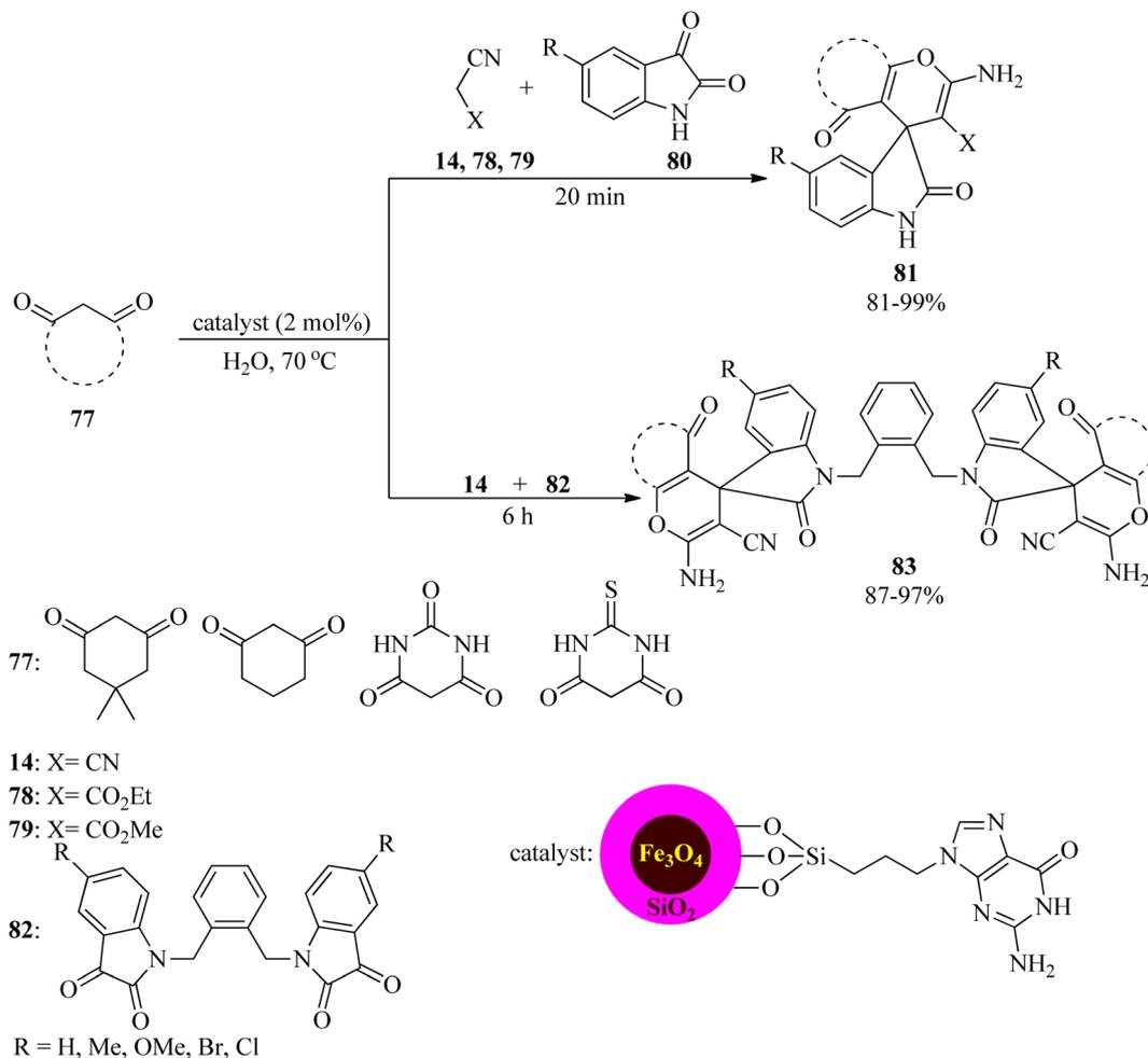
Scheme 25 Preparation of 2',5-dioxo-5,6,7,8-tetrahydrospiro[chromene-4,3'-indoline]-3-carbonitriles and substituted dihydro-2-oxopyrroles.
