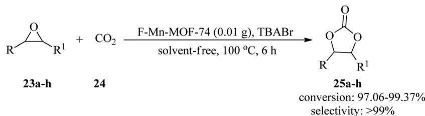
**a:** R = Me, R<sup>1</sup> = H; **b:** R = Et, R<sup>1</sup> = H; **c:** R = -CH<sub>2</sub>Cl, R<sup>1</sup> = H; **d:** R = Ph, R<sup>1</sup> = H; **e:** R = *n*-Bu, R<sup>1</sup> = H;
