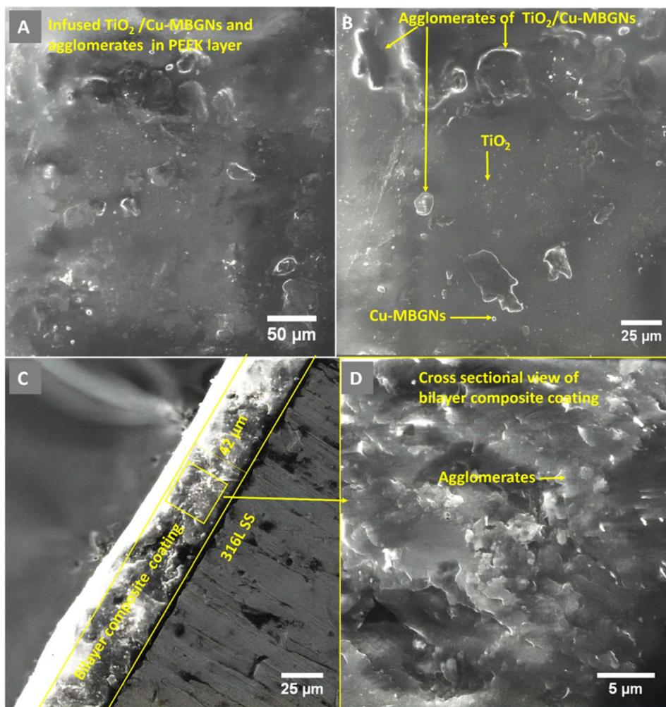
Fig. 3 SEM images of the coating produced at 50 V, 3 min: (A) low magnification showing the deposition of coating; (B) high magnification showing the distribution of TiO<sub>2</sub>/Cu-MBGNs particles on the PEEK layer; (C) cross-section showing coating thickness; and (D) morphology of cross-section of bilayer composite coating.
