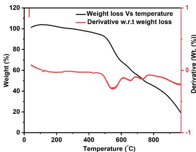
Fig. 8 TGA thermogram for bilayer composite coating.
