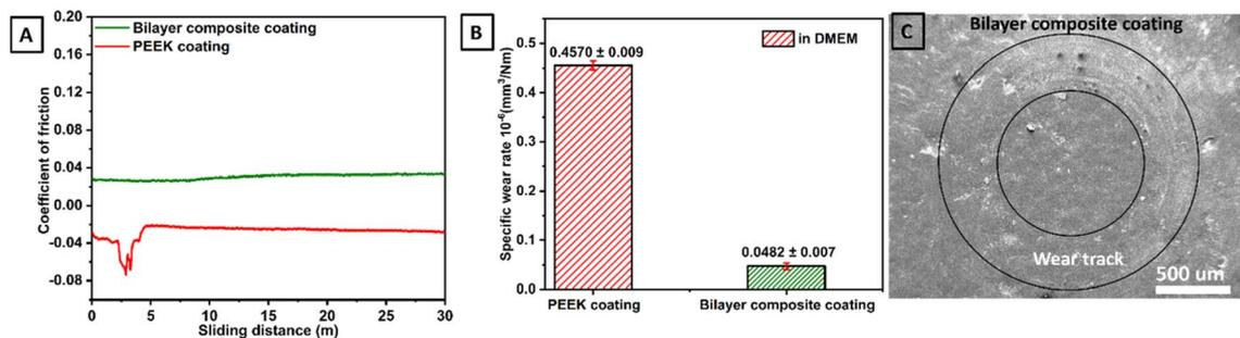
Fig. 14 (A) CoF measured as a function of sliding distance for both PEEK and bilayer composite coatings under wet conditions, *i.e.*, in the presence of DMEM, (B) comparison between specific wear rates and (C) SEM image of wear track of bilayer composite coating.
