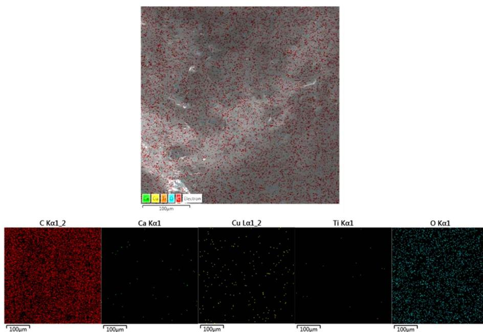
Fig. 5 EDS elemental mapping images, which confirms the presence of  $\text{TiO}_2/\text{Cu-MBGNs}$  in the bilayer composite coating.
