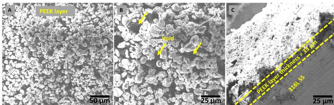
Fig. 2 Morphology of a PEEK layer deposited at 20 V and 1 min, followed by sintering at 350 °C. (A) Shows the morphology of PEEK layer deposited on 316L SS *via* EPD, (B) shows the voids present in PEEK layer, and (C) shows the thickness of PEEK layer.
