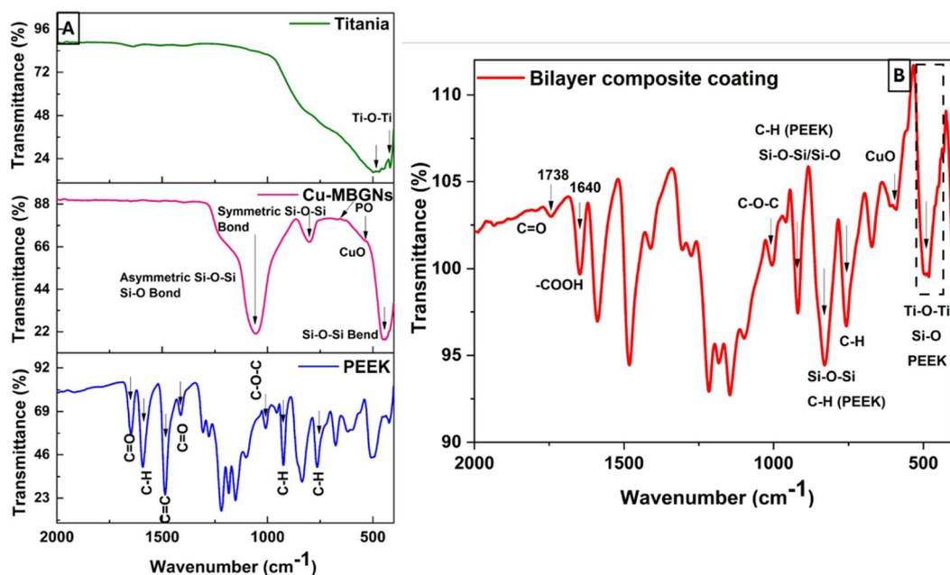
Fig. 6 FTIR spectra of (A) PEEK, Cu-MBGNs, TiO<sub>2</sub>, and (B) bilayer composite coating.
