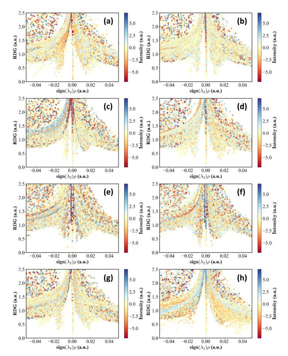
Fig. 10 The RDG  $vs. sign(\lambda_2)\rho(r)$  plots for (a) CO@Al<sub>8</sub>O<sub>12</sub>, (b) CO<sub>2</sub>@Al<sub>8</sub>O<sub>12</sub>, (c) H<sub>2</sub>@Al<sub>8</sub>O<sub>12</sub>, (d) N<sub>2</sub>@Al<sub>8</sub>O<sub>12</sub>, (e) NO@Al<sub>8</sub>O<sub>12</sub>, (f) NO<sub>2</sub>@Al<sub>8</sub>O<sub>12</sub>, (g) O<sub>2</sub>@Al<sub>8</sub>O<sub>12</sub>, (h) SO<sub>2</sub>@Al<sub>8</sub>O<sub>12</sub>. The calculations are performed at  $\omega$ B97XD/Def2-TZVP level of theory.
