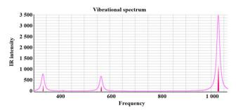
Fig. 2 Vibrational frequency spectrum of the isolated  $Al_8O_{12}$  cluster, displaying all stable (positive) vibrational modes. The x-axis represents the vibrational frequencies (cm $^{-1}$ ), while the y-axis shows the corresponding IR intensities (km mol $^{-1}$ ). Peaks denote distinct vibrational modes, with intensity values reflecting the relative strength of IR absorption. Vibrational frequency calculations are performed at  $\omega$ B97XD/Def2-TZVP level of theory.
