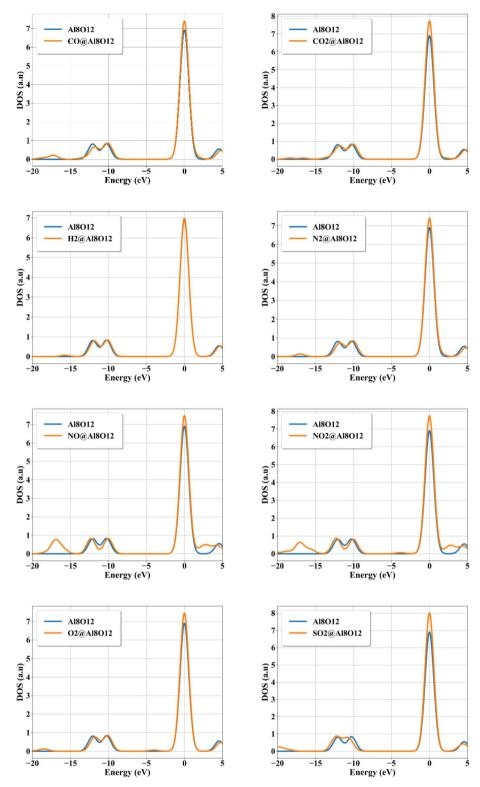
Fig. 6 Total Density of States (TDOS) plot for the  $Al_8O_{12}$  cluster and the adsorbed gases, including CO, CO<sub>2</sub>, H<sub>2</sub>, N<sub>2</sub>, NO, NO<sub>2</sub>, O<sub>2</sub>, and SO<sub>2</sub>. The *x*-axis represents the energy levels (in eV), while the *y*-axis shows the total number of electronic states per energy interval (states per eV). The calculations are performed at  $\omega$ B97XD/Def2-TZVP level of theory.
