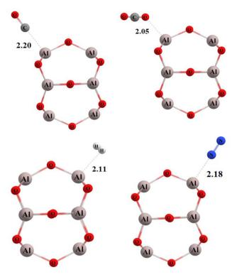
Fig. 4 Optimized structures of gas molecules CO, CO<sub>2</sub>, H<sub>2</sub>, and N<sub>2</sub> adsorbed on the outer surface of the Al<sub>8</sub>O<sub>12</sub> cluster. Calculations were performed at the  $\omega$ B97XD/Def2-TZVP level of theory. Bond lengths are presented in Å.
