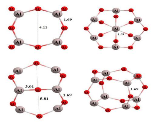
Fig. 1 The optimized structure of the  $Al_8O_{12}$  cluster in different orientations was obtained at  $\omega B97XD/Def2-TZVP$  level of theory. The values of bond length are in Å.
