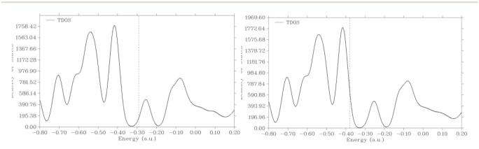
Fig. 15 Schematic diagram of RDX density of states under magnetic fields (0T, 3T, 5T, 6T, 8T, and 12T), with vertical lines representing HOMO energy.
