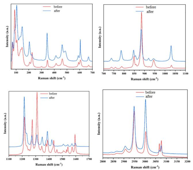
Comparison of Raman spectra of RDX crystals before and after irradiation with  $\pm 6T$  alternating magnetic field
