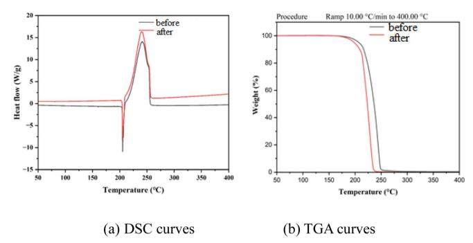
Fig. 11 Thermal performance curves of RDX crystals before and after irradiation with  $\pm 6T$  alternating magnetic field.
