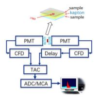
Fig. 4 Structural diagram of positron annihilation lifetime spectrometer.
