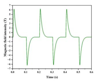
Fig. 3 Variation curve of bidirectional pulse magnetic field intensity over time.
