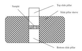
(b) friction sensitivity test
