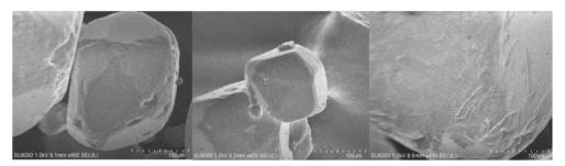
Fig. 7 SEM images of RDX crystals after magnetic field irradiation.
