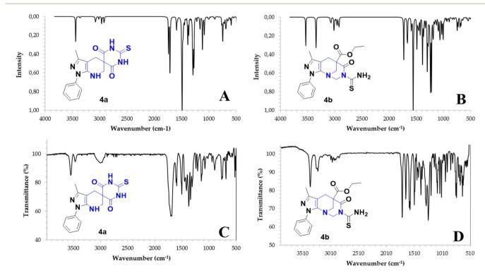
Fig. 2 IR spectra calculated using DFT (B3LYP/6-31G\*) (A and B) and experimental (C and D) IR spectra for 4a and 4b.
