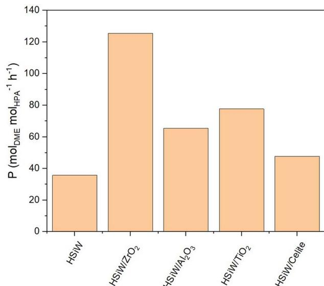
Fig. 7 Productivity  $P_{\text{mol}}$  of HSiW on different supports. Reaction conditions:  $T = 250\text{ }^{\circ}\text{C}$ ,  $p = 50\text{ bar}$ ,  $\text{H}_2/\text{CO}_2\text{ }3/1$ ,  $\text{GHSV} = 10\text{ }000\text{ h}^{-1}$ .
