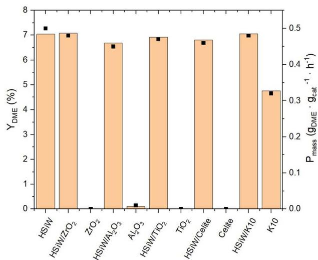
Fig. 6 Yield of DME  $Y_{\text{DME}}$  and productivity  $P_{\text{mass}}$  of HSiW on different supports. Reaction conditions:  $T = 250$  °C,  $p = 50$  bar, H<sub>2</sub>/CO<sub>2</sub> 3/1, GHSV = 10 000 h<sup>-1</sup>.
