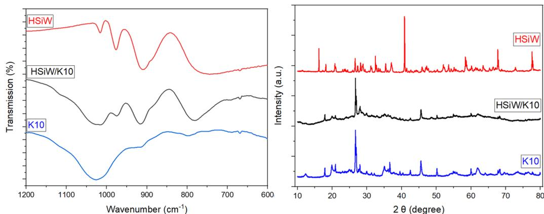
Fig. 2 Exemplary IR spectra (left) and XRD (right) of pure HSiW (red line), HSiW supported on K10 (black line) and pure K10 (blue line).
