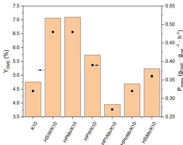
Fig. 4 Yield of DME  $Y_{\text{DME}}$  and productivity  $P_{\text{mass}}$  of HPAs supported on K10. Reaction conditions:  $T = 250\text{ }^\circ\text{C}$ ,  $p = 50\text{ bar}$ ,  $\text{H}_2/\text{CO}_2$  3/1,  $\text{GHSV} = 10\ 000\ \text{h}^{-1}$ .
