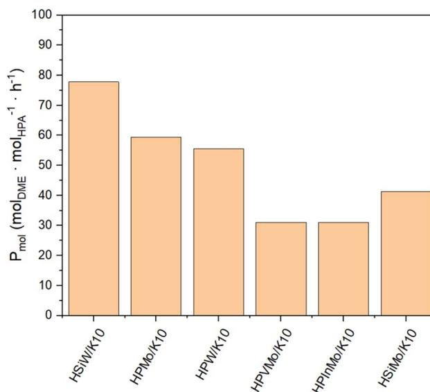
Fig. 5 Productivity  $P_{\text{mol}}$  of HPAs supported on K10. Reaction conditions:  $T = 250$  °C,  $p = 50$  bar,  $\text{H}_2/\text{CO}_2$  3/1, GHSV = 10 000 h<sup>-1</sup>.
