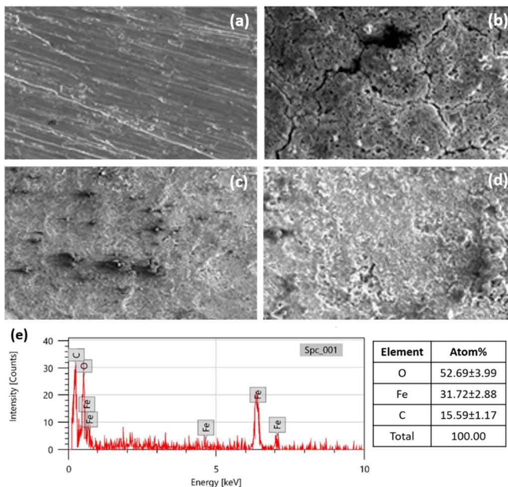
Fig. 9 SEM images of the MS (a) polished chip; (b) immersed in 1 M H<sub>2</sub>SO<sub>4</sub> in the absence of inhibitor for 24 hours; (c) in an open environment with a coating inhibitor, (d) with an inhibitor at a concentration of 400 ppm in 1 M H<sub>2</sub>SO<sub>4</sub> solution for 24 hours, and (e) EDS-SEM images of the MS with an inhibitor at a concentration of 400 ppm in 1 M H<sub>2</sub>SO<sub>4</sub> solution for 24 hours.
