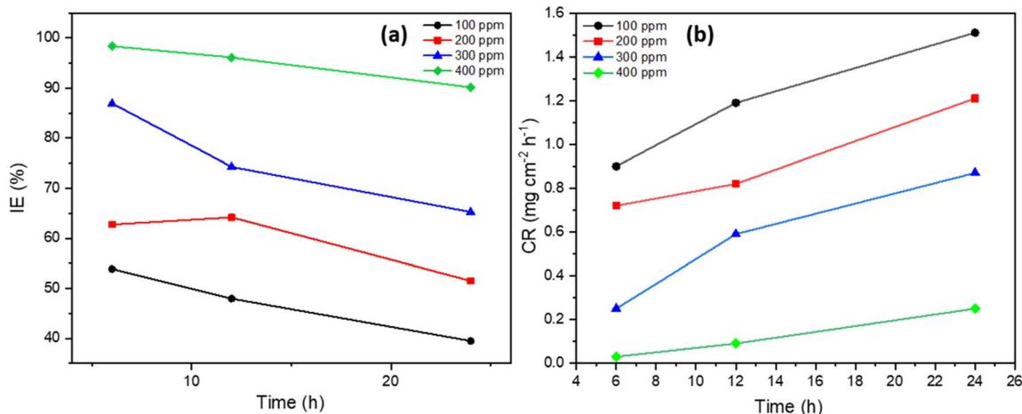
Fig. 2 (a) The inhibition efficiency effect, and (b) the corrosion rate of MS with various concentrations of inhibitor in 1 M H<sub>2</sub>SO<sub>4</sub> solution at 303 K.
