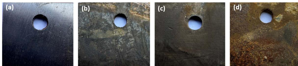
Fig. 10 Images of MS chips (a) fresh MS chips, (b) in an open environment with a coating of the inhibitor, (c) in the presence of the inhibitors with 400 ppm concentration in 1 M H<sub>2</sub>SO<sub>4</sub> solution, and (d) in 1 M H<sub>2</sub>SO<sub>4</sub> solution.
