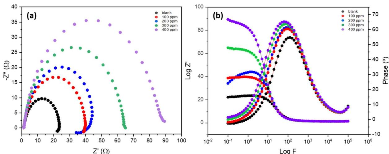
Fig. 5 (a) Nyquist plots, and (b) Bode plots for MS in 1 M H<sub>2</sub>SO<sub>4</sub> solution with and without inhibitor at 303 K. Results are normalized by the exposed surface area of the MS sample.
