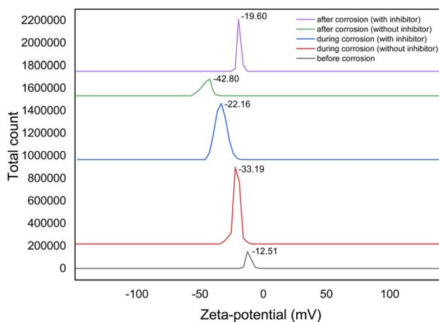
Fig. 11 Zeta-potential graph for MS in 1 M H<sub>2</sub>SO<sub>4</sub> solution at 303 K, before, during and after corrosion, both with and without at 400 ppm concentration of *Rumex nepalensis* inhibitor.
