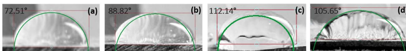
Fig. 7 The contact angle of MS chips (a) fresh MS chip, (b) in an open environment with a coating inhibitor, (c) in the presence of inhibitor (at a concentration of 400 ppm) in 1 M  $\text{H}_2\text{SO}_4$  solution, and (d) in 1 M  $\text{H}_2\text{SO}_4$  solution.
