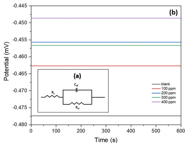
Fig. 4 (a) Equivalent circuit used to fit impedance data of mild steel in 1 M H<sub>2</sub>SO<sub>4</sub> solution with and without inhibitor at 303 K, (b) OCP versus time curves for mild steel in 1 M H<sub>2</sub>SO<sub>4</sub> solution with and without inhibitor at 303 K.
