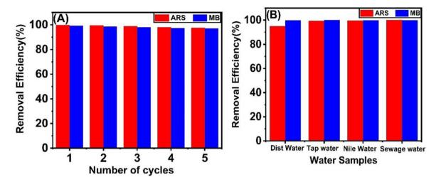
(A) The reusability of SAC adsorbent for MB and ARS dyes; (B) removal of MB and ARS from real water samples using SAC adsorbent.
