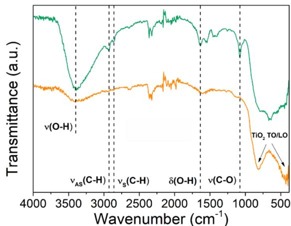
Fig. 5 ATR-FTIR spectra of the as-deposited (green line) Ti–EG and air-annealed Ti–EG-a (orange line) thin films deposited on Si/SiO<sub>2</sub> substrates grown at  $105\text{ }^\circ\text{C}$  after 600 ALD/MLD cycles.
