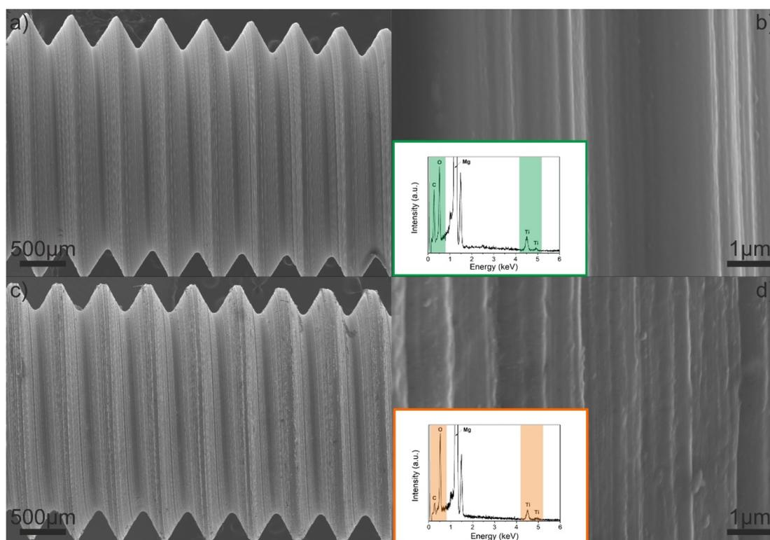
Fig. 7 Top-view SEM images of (a and b) as-deposited Ti-EG and (c and d) air-annealed Ti-EG-a thin films deposited on the AZ31 screw-like substrate grown at 105 °C after 600 ALD/MLD cycles. The insets reveal the EDX spectra.
