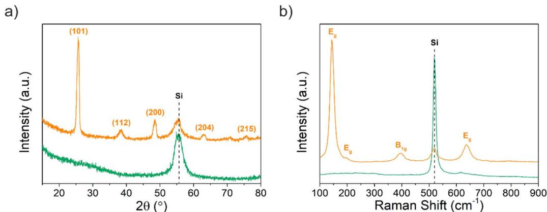
Fig. 4 (a) GIXRD pattern and (b) Raman spectra of the as-deposited (green line) Ti-EG and air-annealed Ti-EG-a (orange line) thin films deposited on Si/SiO<sub>2</sub> substrates grown at 105 °C after 600 ALD/MLD cycles. The observed broad reflection at 50–60° is assigned to the characteristic (311) plane of the crystalline Si(100) substrate.
