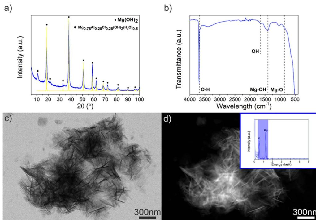
Fig. 10 (a) Powder XRD pattern and (b) ATR-FTIR spectrum (c) TE-STEM mode image and (d) the corresponding ZC-STEM mode image of the degradation products ( $\text{Mg}(\text{OH})_2$ ). The inset in (d) reveals the EDX spectrum, confirming the presence of O and Mg.
