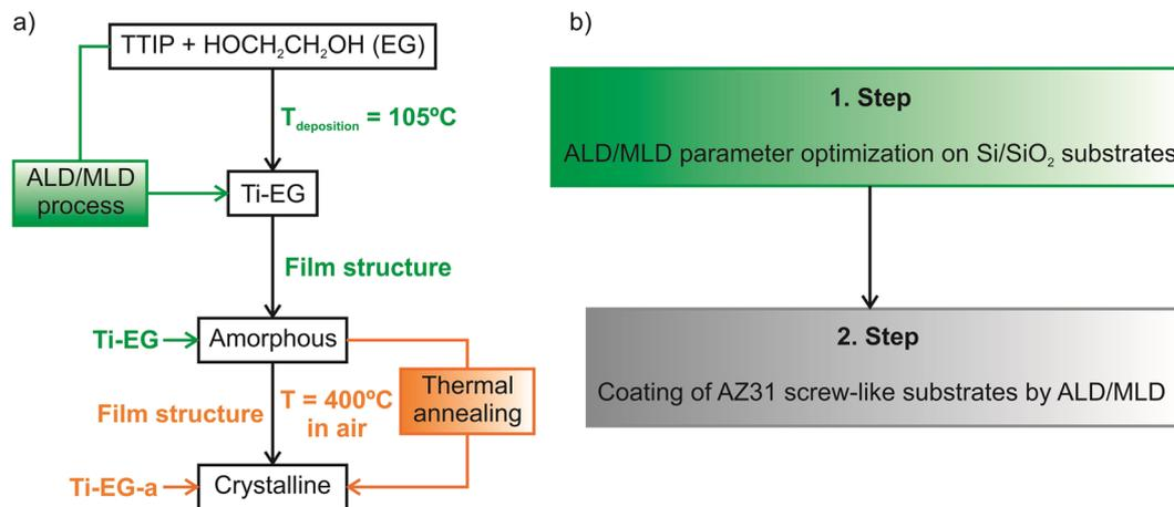
Fig. 2 (a) Schematic of the synthetic procedure for Ti-EG deposition as well as the *ex situ* thermal annealing step. (b) Schematic illustration of the workflow representing the obtained results: (1) Si/SiO<sub>2</sub> and (2) AZ31 screw-like substrates.
