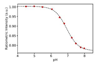
Fig. 4 Response data and response curve for the calibration buffers used to determine the pH of IVF buffers.
