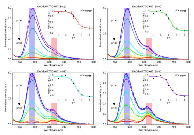
Fig. 3 Fluorescence emission spectra of pH titrations ( $\lambda_{Ex} = 510$  nm), showing the effect of changing the DAOTA/ATTO-647 loading ratio on emission spectra and response curves (insets). The response curves were calculated as the ratio between the summed response signal (blue area) and the summed reference signal (red area), emulating the emission bands that were used during plate reader measurements. Error bars are calculated from the instrumental response error.
