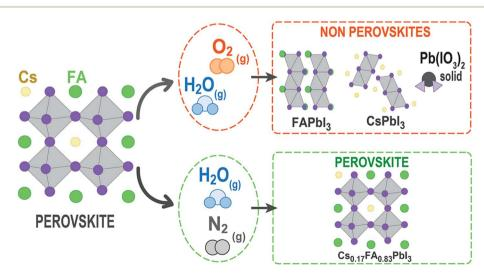
Fig. 6 Degradation of FA based perovskite through vacancy formation, iodide oxidation, and phase segregation into non-perovskite phases under exposure to H<sub>2</sub>O-N<sub>2</sub> and H<sub>2</sub>O-O<sub>2</sub> environment. Figure reproduced with permission from ref. 71.
