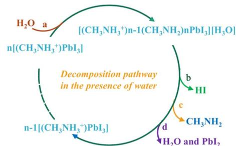
Fig. 3 Decomposition path of perovskites in existence of moisture.<sup>32</sup>
