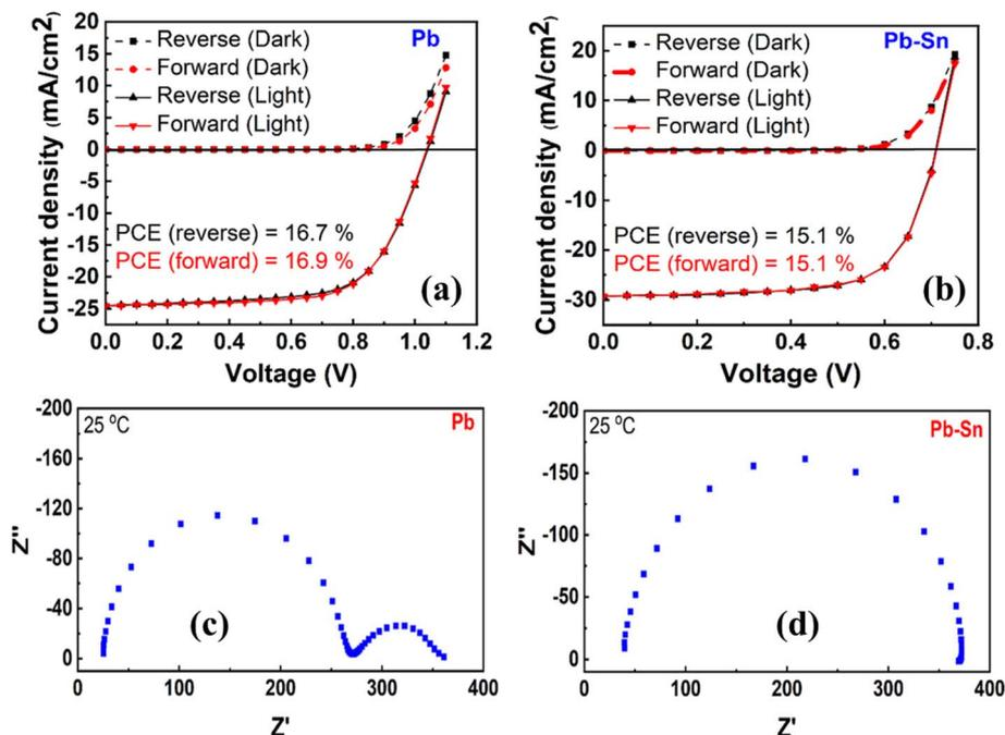
Fig. 14  $J-V$  characteristic (light and dark) of (a) Pb-based PSC (with 2PACz HTL) and (b) Pb-Sn-based PSC (with PEDOT:PSS HTL) with a scan rate of  $100 \text{ mV s}^{-1}$ ; Nyquist plot of (c) a Pb-based PSC and (d) a Pb-Sn-based PSC recorded under irradiation with a 470 nm LED at open circuit and at 25 °C. Figure reprinted with permission from ref. 165.
