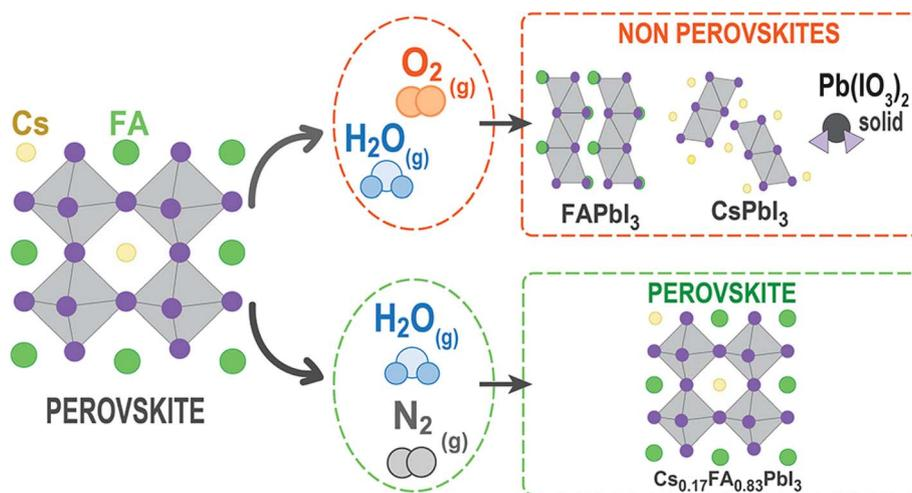
Fig. 6 Degradation of FA based perovskite through vacancy formation, iodide oxidation, and phase segregation into non-perovskite phases under exposure to  $\text{H}_2\text{O-N}_2$  and  $\text{H}_2\text{O-O}_2$  environment. Figure reproduced with permission from ref. 71.
