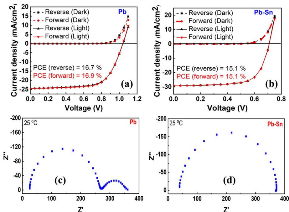
Fig. 14  $J$ - $V$  characteristic (light and dark) of (a) Pb-based PSC (with 2PACz HTL) and (b) Pb-Sn-based PSC (with PEDOT:PSS HTL) with a scan rate of  $100 \text{ mV s}^{-1}$ ; Nyquist plot of (c) a Pb-based PSC and (d) a Pb-Sn-based PSC recorded under irradiation with a 470 nm LED at open circuit and at  $25 \text{ }^\circ\text{C}$ . Figure reprinted with permission from ref. 165.
