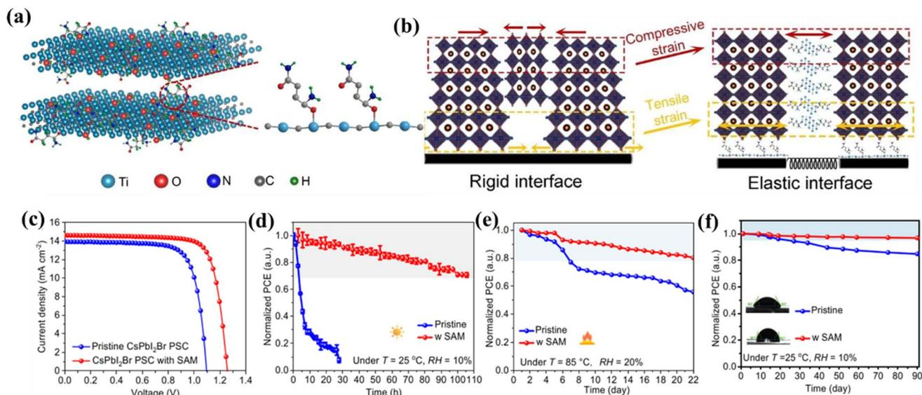
Fig. 13 (a and b) Schematic diagram of alkenamides grafted MXene by forming Ti–O–C bond and residual strain relaxation by forming elastic interface and boundary. (c) Performance of CsPbI<sub>2</sub>Br based PSCs; stability under (d) continuous light irradiation, (e)  $T = 85\text{ }^{\circ}\text{C}$ ,  $\text{RH} = 20\%$  and (f)  $T = 25\text{ }^{\circ}\text{C}$ ,  $\text{RH} = 10\%$  conditions.
