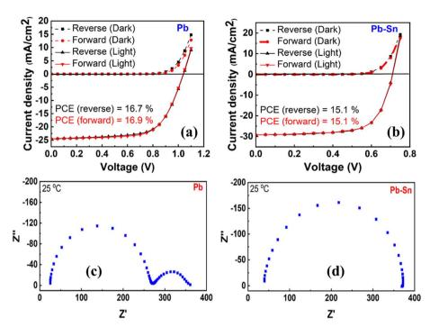
Fig. 14 J-V characteristic (light and dark) of (a) Pb-based PSC (with 2PACz HTL) and (b) Pb-Sn-based PSC (with PEDOT:PSS HTL) with a scan rate of 100 mV s<sup>-1</sup>; Nyquist plot of (c) a Pb-based PSC and (d) a Pb-Sn-based PSC recorded under irradiation with a 470 nm LED at open circuit and at 25 °C. Figure reprinted with permission from ref. 165.
