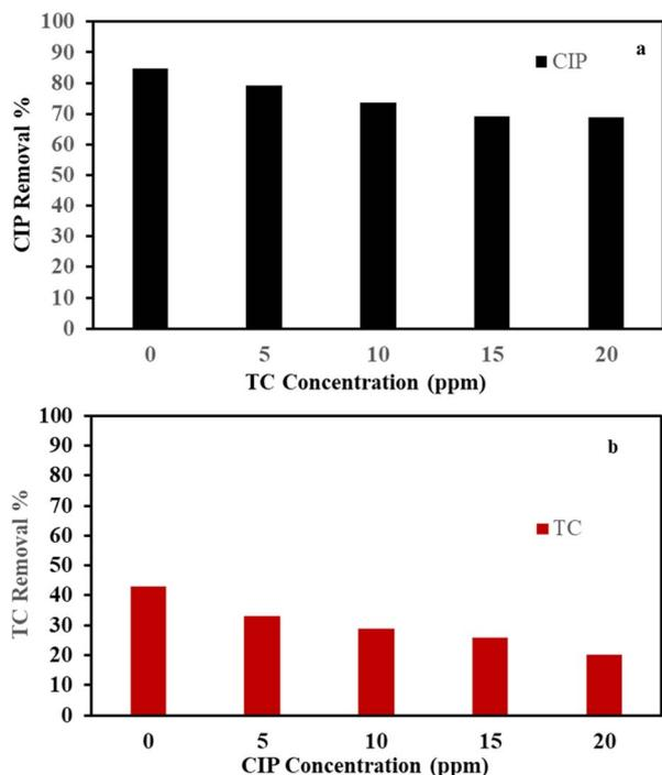
Fig. 9 Removal of CIP in presence of 0–20 mg L<sup>-1</sup> TC (a) removal of TC in presence of 0–20 mg L<sup>-1</sup> CIP (b).
