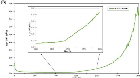
Fig. 14 Thermal diffusivity ( $\alpha$ ) values of (cell-4/CF/PEG) with alteration in: (A) temperature and (B) time
