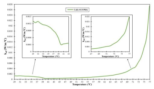
Fig. 17 Effective thermal conductivity coefficient ( $k_{eff}$ ) values of (cell-4/CF/PEG) with temperature alteration
