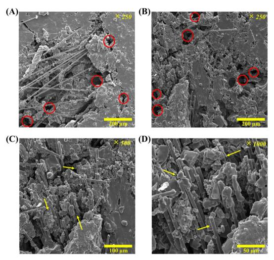
Fig. 18 FESEM micrographs of (cell-4/CF/PEG) in: (A) and (B)  $\times$ 250 magnification and 200  $\mu$ m scale, (C)  $\times$ 500 magnification and 100  $\mu$ m scale and (D)  $\times$ 1000 magnification and 50  $\mu$ m scale.
