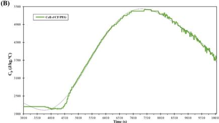
Fig. 16 Specific heat capacity ( $C_p$ ) values of (cell-4/CF/PEG) with alteration in: (A) temperature and (B) time.
