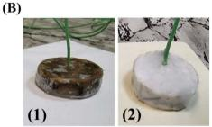
Fig. 2 Time-temperature history analysis set-up in: (A) heating and cooling cycle and (B) image of prepared (cell-4/CF/PEG) (1) and (cell-4/CF/ SR) (2) samples incorporated with thermocouples.
