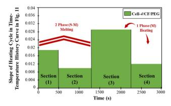
Fig. 12 Thermal diffusivity ( $\alpha$ ) index of (cell-4/CF/PEG)
