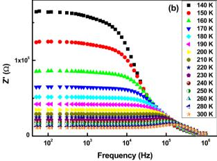
Fig. 11 Evolution of the real part of the impedance Z' as a function of frequency at different temperatures for the samples (a) RF/VOX-625 and (b) RF/VOX-650.
