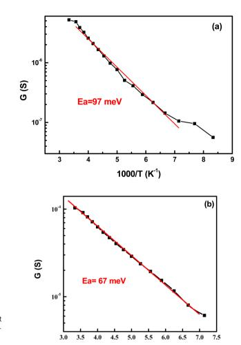
Fig. 10 Variation of AC conductance as a function of temperature for samples (a) RF/VOX-625 and (b) RF/VOX-650.
