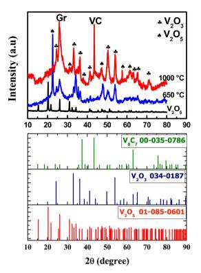
Fig. 1  $\,$  XRD pattern of the  $\rm V_2O_5$  nanopowder and the nanocomposite RF/VOX pyrolyzed at 650 °C and 1000 °C.
