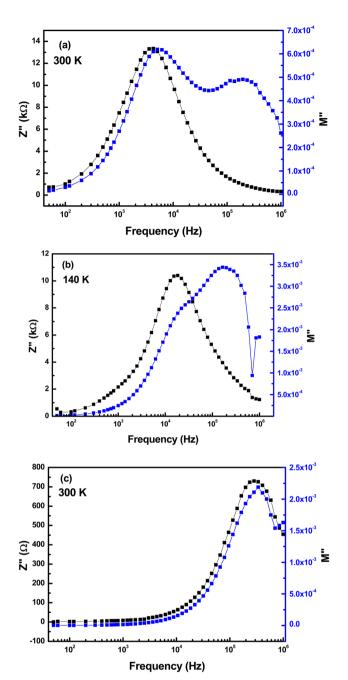
Fig. 16 Variation of combined M'' and Z'' as a function of frequency for the nanocomposites (a) RF/VOX-625 at T = 300 K, (b) RF/VOX-650 at T = 140 K and (c) RF/VOX-650 at T = 300 K.
