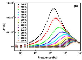
Fig. 12 Frequency dependence of the imaginary part of impedance Z'' at different temperatures for samples (a) RF/VOX-625 and (b) RF/VOX-650.
