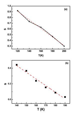
**Fig. 9** Linear part of the exponent s as a function of the measurement temperature for the nanocomposites (a) RF/VOX-625 and (b) RF/VOX-650.
