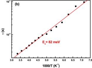
Fig. 13 Evolution of the relaxation time according to the Arrhenius law of the nanocomposites (a) RF/VOX-625 and (b) RF/VOX-650.
