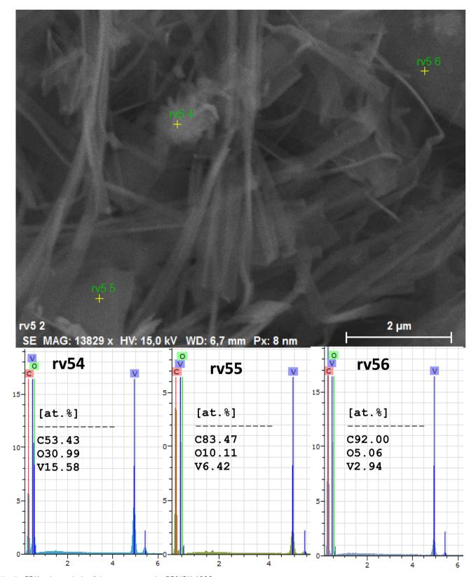
Fig. 5 EDX point analysis of the nanocomposite RF/VOX-1000.
