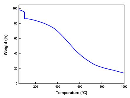
Fig. 6 TGA curve of the RF/VOX nanocomposite.
