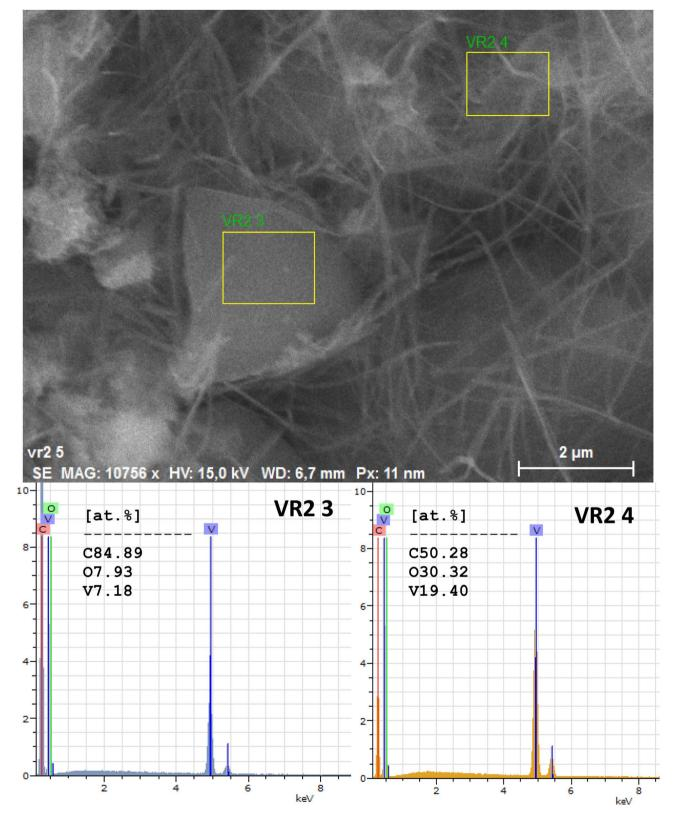
Fig. 4 EDX point analysis of the nanocomposite RF/VOX-650
