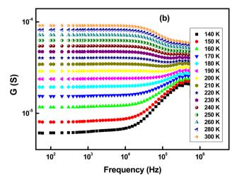
Fig. 7 Variation of conductivity as a function of frequency at different temperatures for (a) RF/VOX-625 and (b) RF/VOX-650 nanocomposites.
