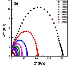
Fig. 14 Nyquist diagram of (a) RF/VOX-625 and (b) RF/VOX-650 nanocomposites.
