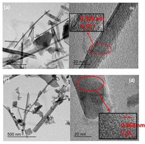
Fig. 2 TEM micrographs of the nanocomposites: (a and b) RF/VOX-650 and (c and d) RF/VOX-1000
