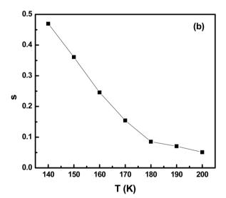
Fig. 8 Variation of exponent s with temperature for (a) RF/VOX-625 and (b) RF/VOX-650 nanocomposites.
