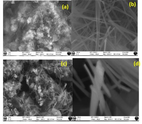
Fig. 3 SEM micrographs of the nanocomposites: (a and b) RF/VOX-650 and (c and d) RF/VOX-1000.
