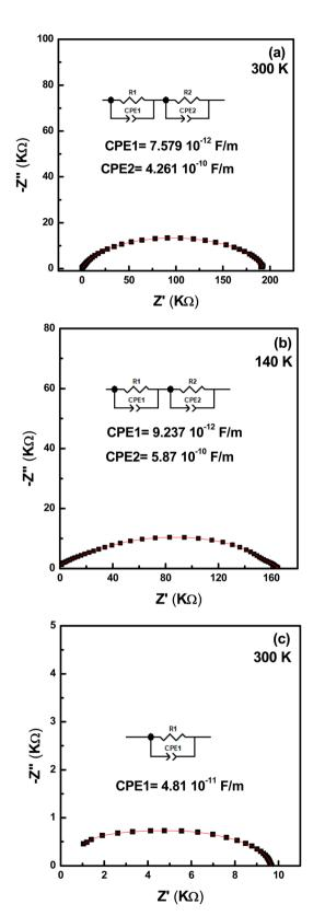
Fig. 15 Fitting of the Nyquist diagrams using the Zview software for samples (a) RF/VOX-625 at T = 300 K, (b) RF/VOX-650 at T = 140 K and (c) RF/VOX-650 at T = 300 K.
