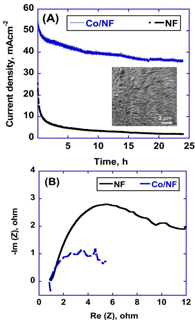
Fig. 5 (A) Chronoamperometry measurement @  $0.5\text{ V}$  using NF and Co/NF, and (B) EIS of bare NF and Co/NF using  $0.33\text{ M}$  and  $0.5\text{ V}$ . Voltages are vs. Ag/AgCl, and the electrolyte used is 1 M KOH.
