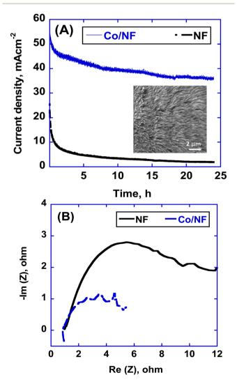
Fig. 5 (A) Chronoamperometry measurement @ 0.5 V using NF and Co/NF, and (B) EIS of bare NF and Co/NF using 0.33 M and 0.5 V. Voltages are vs. Aq/AqCl, and the electrolyte used is 1 M KOH.
