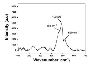
Fig. 3 Raman spectra of Co/NF sample.
