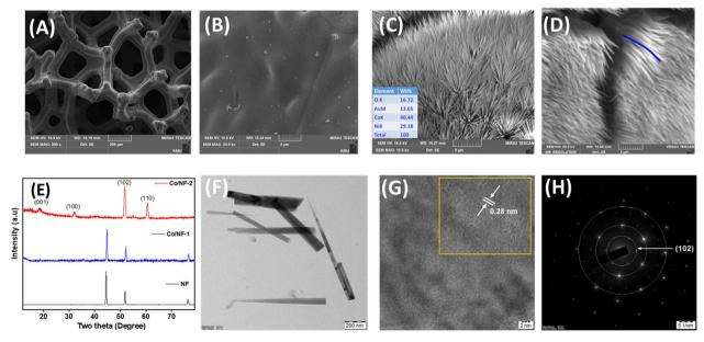
Fig. 1 (A) low-resolution image of NF, (B) high-resolution image of NF, (C and D) high-resolution image of the Co/NF (inset in (C) shows the elemental analysis, while the blue line in (D) shows the length of the nano-grass), (E) XRD of NF, Co/NF-1, and Co/NF-2, (F) TEM images of the Co/NF, (G) HRTEM of the Co/NF, and (H) SAED of Co/NF.
