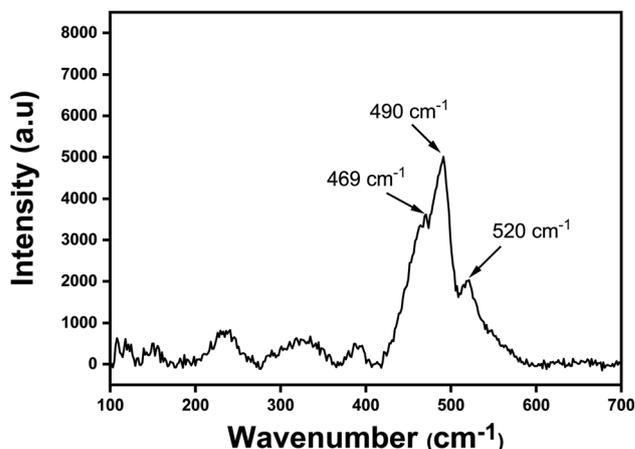
Fig. 3 Raman spectra of Co/NF sample.
