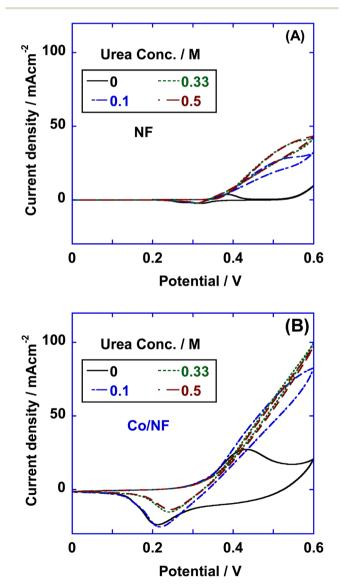
Fig. 4 CV of the bare NF (A) and Co/NF (B) using different urea concentrations @ 20 mV s $^{-1}$ . Voltages are vs. Ag/AgCl, and the electrolyte used is 1 M KOH.
