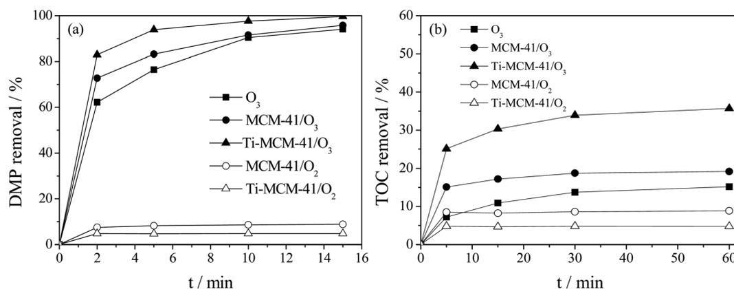
Fig. 7 Comparison of DMP (a) and TOC (b) removal among different processes (initial pH = 5.4, initial DMP concentration = 10 mg L<sup>-1</sup>, catalyst concentration (if use) = 1 g L<sup>-1</sup>, Si/Ti = 80 Ti-MCM-41 (if use)).
