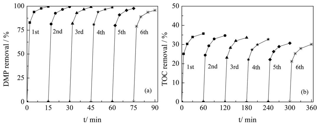
Fig. 8 Activity and stability of Ti-MCM-41 catalyst for ozonation of DMP (a) and TOC (b) (initial pH = 5.4, initial DMP concentration =  $10 \text{ mg L}^{-1}$ , catalyst concentration =  $1 \text{ g L}^{-1}$ ).
