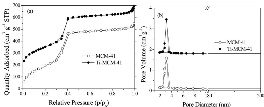
Fig. 4 The N<sub>2</sub> adsorption-desorption isotherms (a) and pore size distribution curves (b) of different catalysts.
