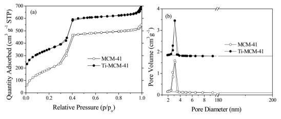
Fig. 4 The N<sub>2</sub> adsorption-desorption isotherms (a) and pore size distribution curves (b) of different catalysts
