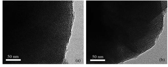
Fig. 2 TEM images of MCM-41 (a) and Ti-MCM-41 (b) catalysts
