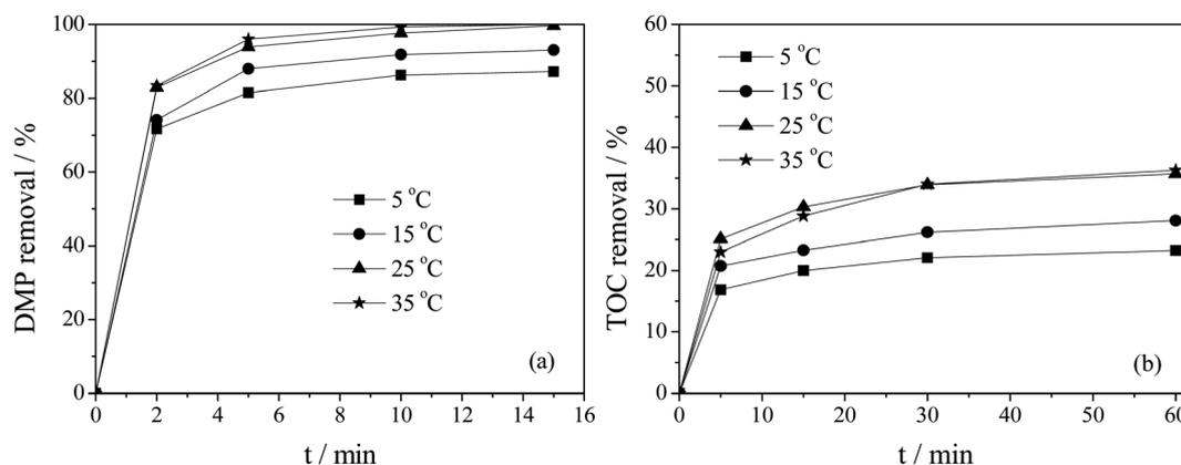
Fig. 6 Effect of reaction temperature on DMP (a) and TOC (b) removal (initial pH = 5.4, initial DMP concentration = 10 mg L<sup>-1</sup>, catalyst concentration = 1 g L<sup>-1</sup>, Si/Ti = 80 Ti-MCM-41).
