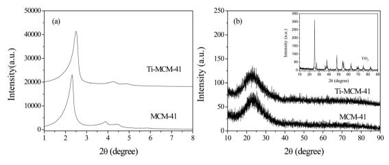
Fig. 1 Low angle (a) and wide-angle (b) XRD patterns of different catalyst samples.
