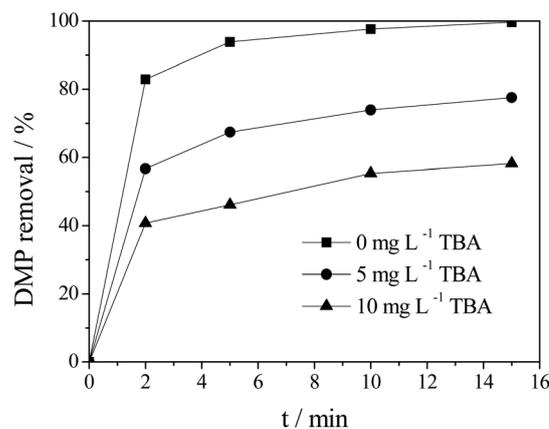
Fig. 10 Influence of TBA in catalytic ozonation of DMP over Ti-MCM-41 (initial pH = 5.4, initial DMP concentration =  $10 \text{ mg L}^{-1}$ , catalyst concentration =  $1 \text{ g L}^{-1}$ , Si/Ti = 80 Ti-MCM-41).
