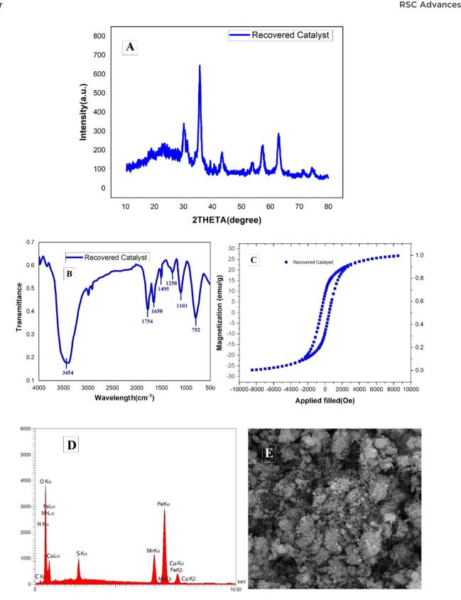
$\label{eq:Fig. 10 (A) XRD, (B) FT-IR, (C) VSM, (D) EDX and, (E) SEM analysis of the recovered MCFe_2O_4@Alginate@SAA and (E) SEM and$
