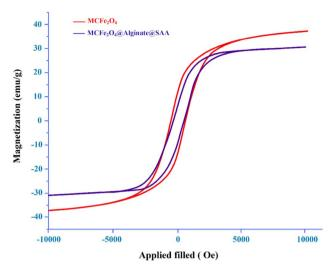
Fig. 4 VSM diagrams of MCFe<sub>2</sub>O<sub>4</sub> and MCFe<sub>2</sub>O<sub>4</sub>@Alginate@SAA.
