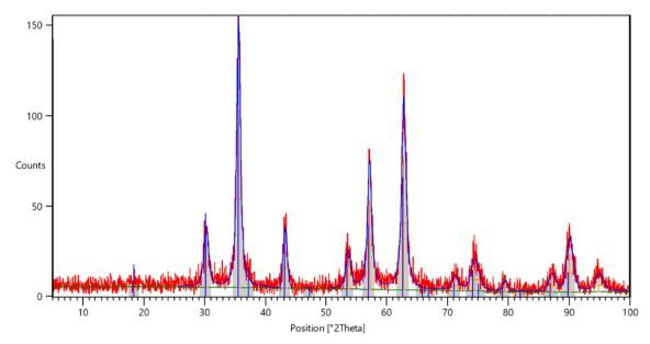
Fig. 3 XRD spectra of MCFe<sub>2</sub>O<sub>4</sub>@Alginate@SAA.
