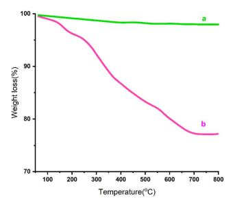
Fig. 5 TGA spectra of (a) MCFe<sub>2</sub>O<sub>4</sub> and (b) MCFe<sub>2</sub>O<sub>4</sub>@Alginate@SAA
