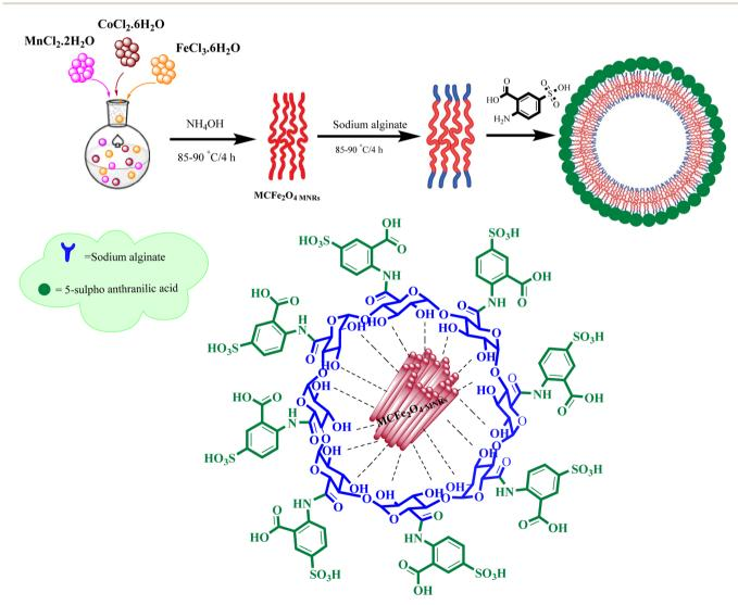
Scheme 1 Synthesis of MCFe<sub>2</sub>O<sub>4</sub>@Alginate@SAA.
