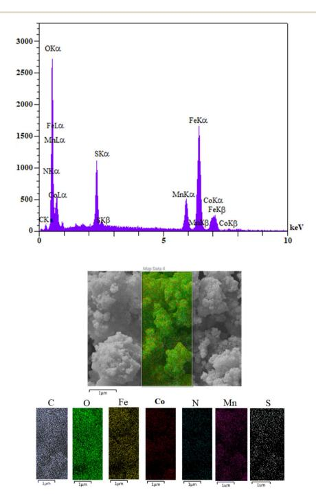
Fig. 7 EDAX spectra of MCFe<sub>2</sub>O<sub>4</sub>@Alginate@SAA and the corresponding EDX elemental mapping pattern of the MCFe<sub>2</sub>O<sub>4</sub>@Alginate@SAA MNRs.
