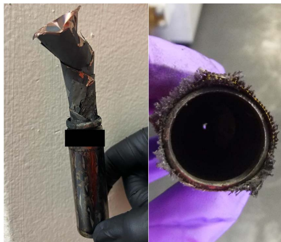
Fig. 7 Comparison of two A-4 cells after failure by external heating at 50% SoC (left, side aspect) and 100% SoC (right, vertical aspect).
