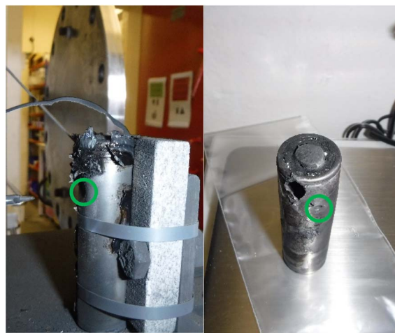
Fig. 8 Images of the effects of cell failure after an A-4 NP test, the green circle indicates the point of entry of the nail.
