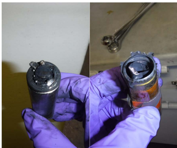
Fig. 6 Comparison of two A-3i cells after failure by external heating at 67% SoC (left) and 100% SoC (right).
