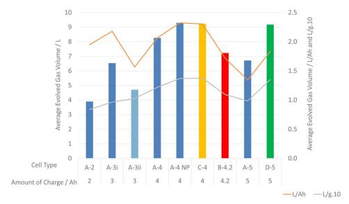
Fig. 2 Graph of average volume of gas evolved for each cell at 100% SoC, with volume also expressed in terms of L Ah<sup>-1</sup> and as a function of the typical mass of each cell, (L  $q^{-1}$ ) × 10.
