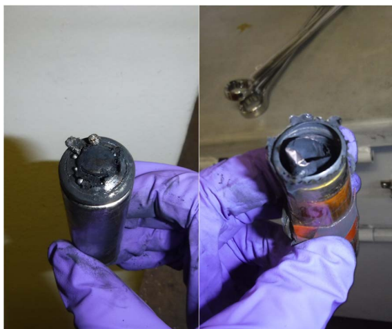
Fig. 6 Comparison of two A-3i cells after failure by external heating at 67% SoC (left) and 100% SoC (right).
