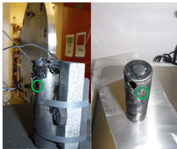
Fig. 8 Images of the effects of cell failure after a A-4 NP test, the green circle indicates the point of entry of the nail.
