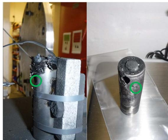
Fig. 8 Images of the effects of cell failure after an A-4 NP test, the green circle indicates the point of entry of the nail.
