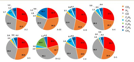
Fig. 4 Pie chart showing the relative amount of CO<sub>2</sub>, H<sub>2</sub>, CO, C<sub>2</sub>H<sub>6</sub>, C<sub>2</sub>H<sub>4</sub>, C<sub>3</sub>H<sub>8</sub>, C<sub>3</sub>H<sub>6</sub> and CH<sub>4</sub> for each of the cells at 100% SoC.
