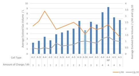
Fig. 3 Graph of average evolved volume of gas for each cell from manufacturer A and L Ah<sup>-1</sup> and (L  $\alpha^{-1}$ )  $\times$  10.
