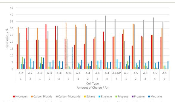
Fig. 5 Graph of relative gas composition for all cells from manufacturer A at each SoC tested, bars for A-3ii are hatched as they are results from previous work.<sup>25</sup>
