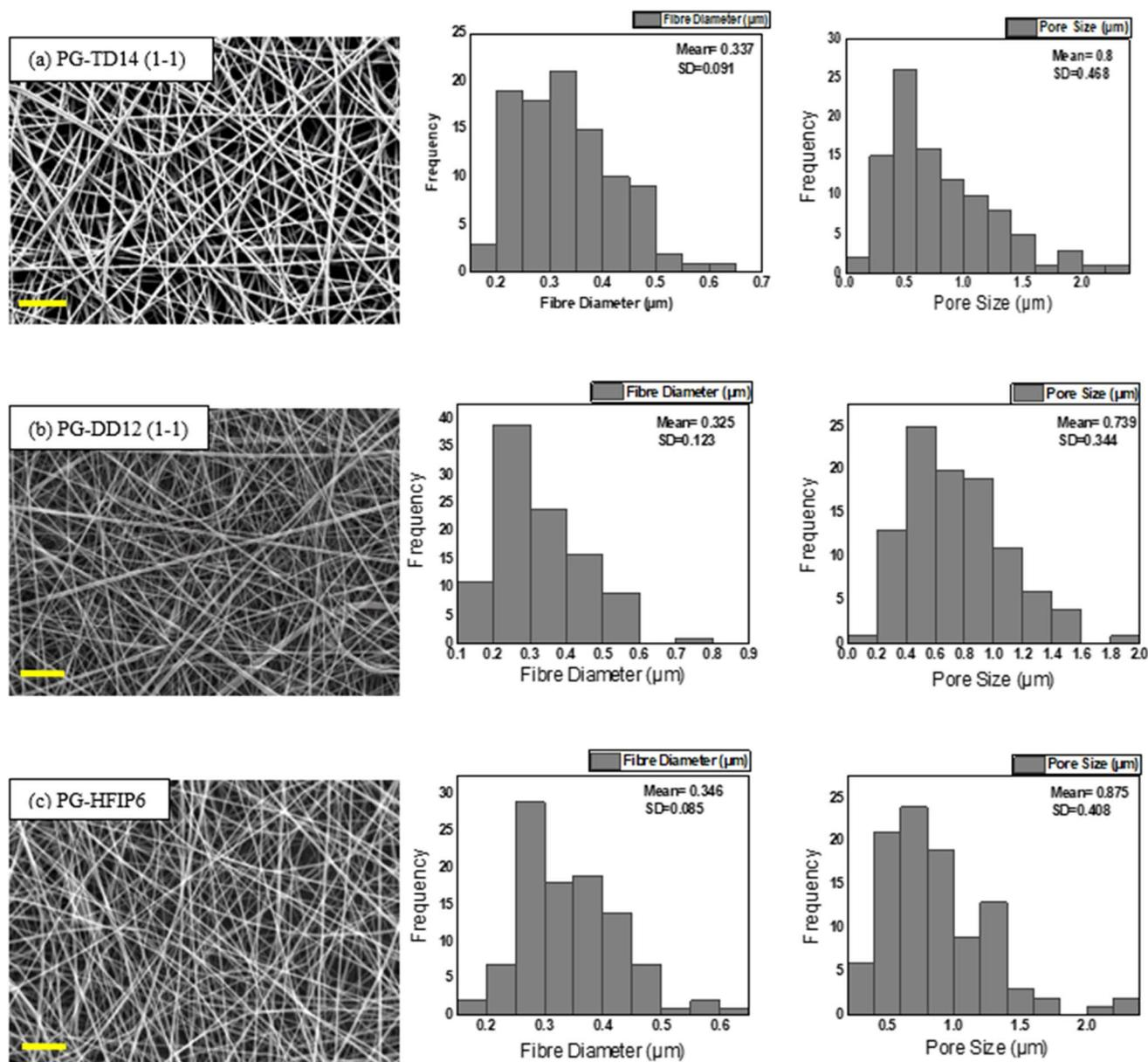
Fig. 7 SEM images of PLGA scaffolds produced from different solvent systems and their corresponding fibre diameter and pore size; (a) 14 w/w% THF-DMF (1-1), (b) 12 w/w% DCM-DMF (1-1), (c) 6 w/w% HFIP; scale bar: 10  $\mu\text{m}$ .
