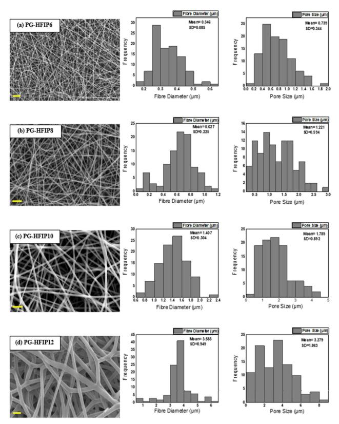
Fig. 4 SEM images and corresponding fibre diameter and pore size distribution graphs of PLGA scaffolds produced from differently concentrated solutions from HFIP including (a) 6 w/w%, (b) 8 w/w%, (c) 10 w/w%, (d) 12 w/w%; scale bar: 10  $\mu$ m.
