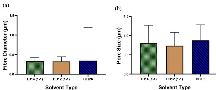
Fig. 8 Comparison of (a) average fibre diameter and (b) pore size for scaffolds from different solvent systems; (\*\*\*)  $P < 0.001$ ,  $N = 5$ ).
