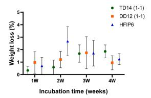
Fig. 13 Degradation profiles of electrospun PLGA scaffolds prepared from various solvent systems over a period of 4 weeks.
