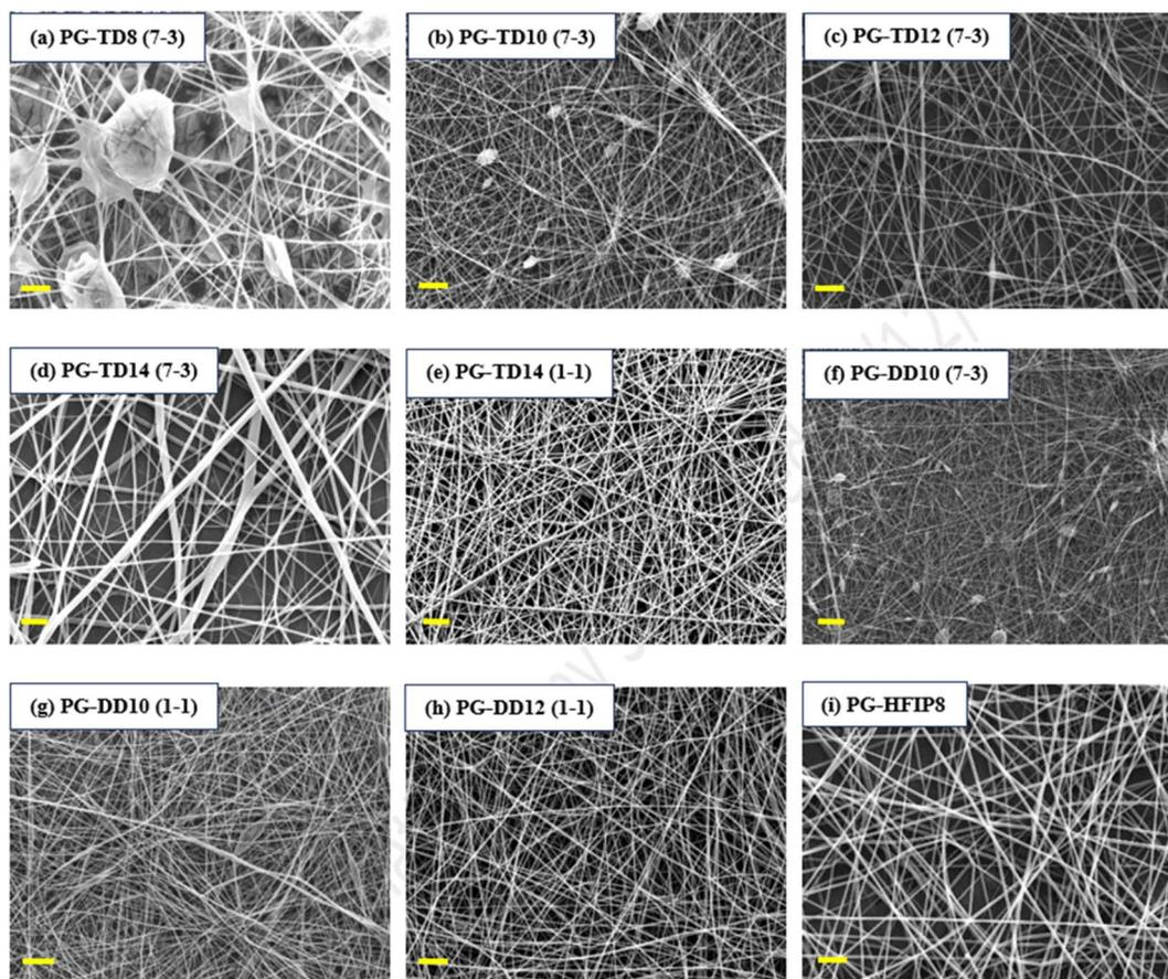
Fig. 3 SEM images of the electrospun PLGA fibres produced from different solvent systems including (a) 8 w/w% THF-DMF (7-3), (b) 10 w/w% THF-DMF (7-3), (c) 12 w/w% THF-DMF (7-3), (d) 14 w/w% THF-DMF (7-3), (e) 14 w/w% THF-DMF (1-1), (f) 10 w/w% DCM-DMF (7-3), (g) 10 w/w% DCM-DMF (1-1), (h) 12 w/w% DCM-DMF (1-1), (i) 10 w/w% HFIP; scale bar: 10  $\mu$ m.
