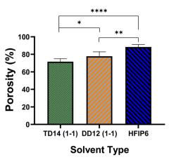
Fig. 12 The porosity of electrospun PLGA scaffolds prepared from various solvent systems; (\*P < 0.05, \*\*P < 0.001, \*\*\*P < 0.001, N = 5).
