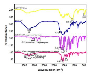
Fig. 2 FT-IR spectrum of raw and intermediate materials and the final structure of the catalyst: (a)  $N^2$ , $N^4$ , $N^6$ -tris(4-(aminomethyl) benzyl)-1,3,5-triazine-2,4,6-triamine, (b) 2,4,6-tris(4-formylphenoxy)-1,3,5-triazine, (c) TPT-TAT, (d) TPT-TAT/silica.
