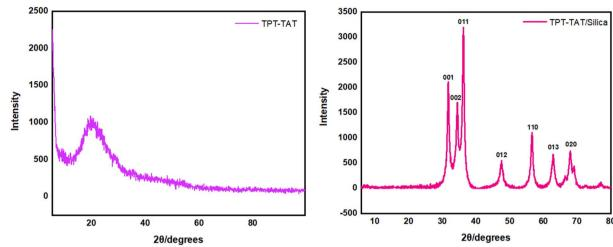
Fig. 7 X-ray diffraction (XRD) pattern of the TPT-TAT/silical
