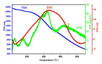
Fig. 8 Thermogravimetric (TG), differential thermal analysis (DTA), and derivative thermogravimetric (DTG) graph of the TPT-TAT/silica, illustrating thermal stability and decomposition behavior.
