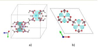
Fig. 1 Primitive unit cell structure of MIL-88A(M), where M (cyan), O (red), C (brown), and H (grey). The red, green, and blue arrows represent the directions of the a, b, and c dimensions along the x, y, and z axes, respectively. (a) Three-dimensional view. (b) Two-dimensional (top) view.
