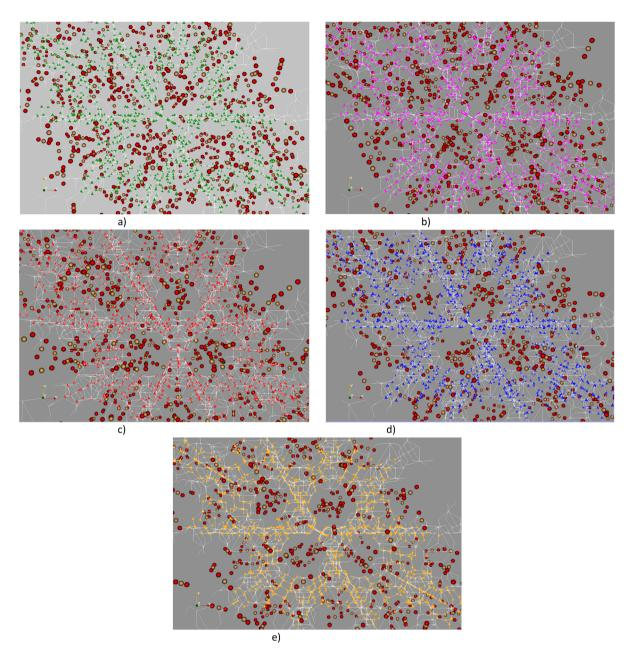
Fig. 6 Visualization of CO<sub>2</sub> adsorption in MIL-88A(M) at 1 bar. At this low pressure, the distribution of gas molecules distributed within the pores of the MOF is primarily governed by adsorption phenomena. (a) CO<sub>2</sub>@MIL-88A(Al). (b) CO<sub>2</sub>@MIL-88A(Gc). (c) CO<sub>2</sub>@MIL-88A(Sc). (d) CO<sub>2</sub>@MIL-88A(Sc). 88A(Ti). (e)  $CO_2@MIL-88A(V)$ .
