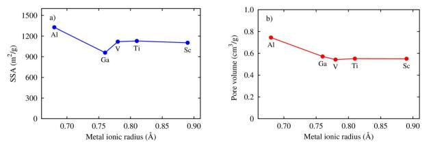
Fig. 8 Relationship between the specific surface area (SSA) and (a) the pore volume (b) the metal ionic radii.
