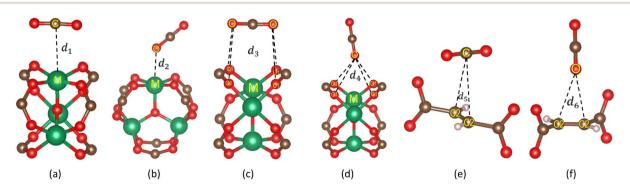
Fig. 5 Favourable adsorption sites and configurations of the  $CO_2$  molecule in MIL-88A(M) with M = Al, Ga, Sc, Ti, and V, where M (green), O (red), C (brown), and H (light pink). (a) Side-on metal. (b) End-on metal. (c) Side-on hollow. (d) End-on hollow. (e) Side-on linker. (f) End-on linker
