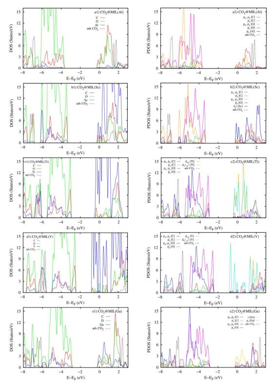
Fig. 11 Atomic projected density of states (the left panels) and orbital projected density of states (the right panels) for the  $CO_2@MIL-88A(M)$  systems with M = Al, Sc, Ti, V, and Ga.
