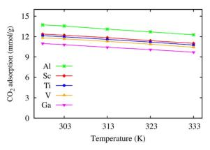
Fig. 4 Temperature dependence of the excess gravimetric loading of  $CO_2$  in MIL-88A(M) at the saturated pressure of 20 bar for M = Ga and 25 bar for the other metal substitutions.
