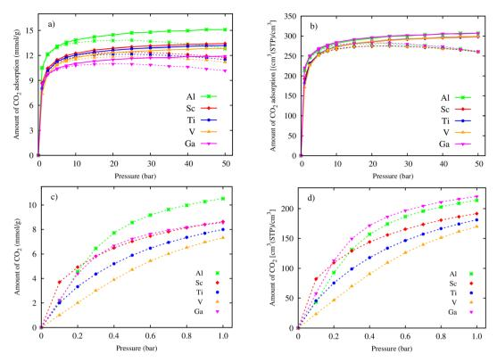
Fig. 3 Excess (dashed lines) and absolute (solid lines)  $CO_2$  adsorption isotherms of MIL-88A(M), where M = Al, Ga, Sc, Ti, and V: (a) gravimetric uptake and (b) volumetric uptake for pressures of up to 50 bar. Zoom-in for gravimetric (c) and volumetric (d)  $CO_2$  adsorption isotherms at low pressures (0–1.0 bar).
