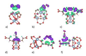
Fig. 9 Charge density difference of the  $CO_2@MIL-88A(Al)$  system at the favourable adsorption sites. Green and violet colours describe the positive and negative charge clouds, respectively. The isosurface value is 0.0003 e Bohr $^{-3}$  isosurface. A similar charge cloud distribution was also found for MIL-88A (Sc, Ti, Vi, and Ga). (a) Side-on metal. (b) Endon metal. (c) Side-on hollow. (d) End-on hollow. (e) Side-on linker. (f) End-on linker.
