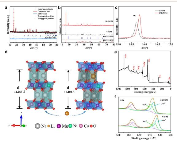
Fig. 2 Material characterization of NNCM and [NL]NCM: (a) Rietveld refinement results of the [NL]NCM powder (b) XRD patterns of the pristine NNCM and [NL]NCM (c) magnified patterns of the two samples between 15° and 17°. (d) Schematic of the effect of Li doping on the electrode structure (e) XPS full spectrum of [NL] NCM and (f) Mn 2p XPS fitted spectra of NNCM and [NL]NCM powders.
