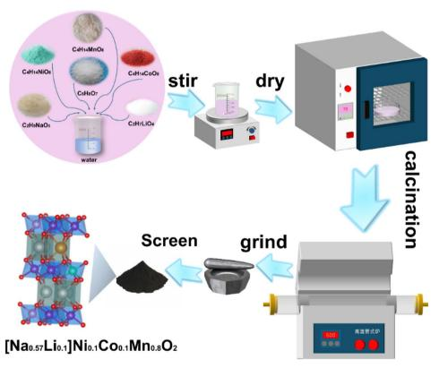
Fig. 1 Synthesis process of the [Na<sub>0.57</sub>Li<sub>0.1</sub>]Ni<sub>0.1</sub>Co<sub>0.1</sub>Mn<sub>0.8</sub>O<sub>2</sub> cathode material
