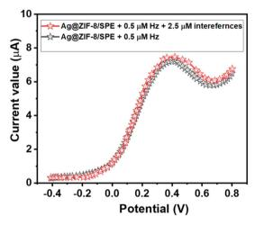
Fig. 5 LSV curves of the Ag@ZIF-8/SPE for 0.5  $\mu$ M hydrazine and 0.5  $\mu$ M hydrazine + 2.5  $\mu$ M interferences (glucose, hydrogen peroxide, ascorbic acid, *para*-nitrophenol, Cl<sup>-</sup>, Na<sup>+</sup>, uric acid, urea, citric acid, and ammonia) at a scan rate of 25 mV s<sup>-1</sup>.
