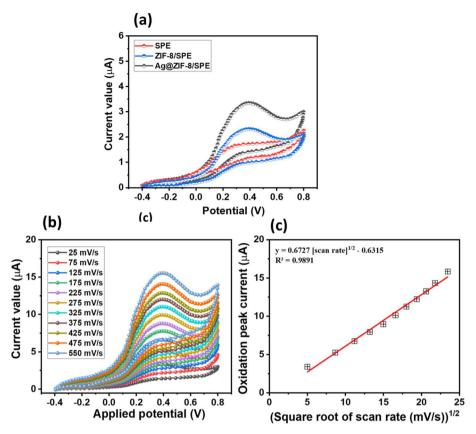
Fig. 3 (a) CV curves of the SPE, ZIF-8/SPE, and Ag@ZIF-8/SPE in the presence of 0.5  $\mu$ M hydrazine (0.1 M PBS, pH = 7.0) under an applied potential scan rate of 25 mV s<sup>-1</sup> (b) CV curves of the Ag@ZIF-8/SPE for 0.5  $\mu$ M hydrazine in 0.1 M PBS (pH = 7.0) at different applied scan rates of 25–550 mV s<sup>-1</sup>. (c) Calibration plot between the electro-oxidation current peak value and square root of the applied scan rates.
