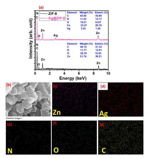
Fig. 2 (a) EDX spectra of ZIF-8 and Ag@ZIF-8. EDX electron image (b), and mapping images for Zn (c), Ag (d), N (e), O (f), and C (g) in the prepared Ag@ZIF-8.
