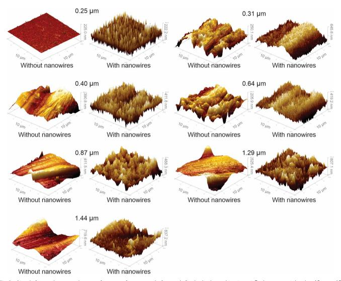
Fig. 2 Atomic force microscopy images of seven surface groups before and after hydrothermal treatment. Each scan was taken in a 10  $\mu$ m  $\times$  10 μm area on the surface. Atomic force microscopy (AFM). Bruker AFM (Bruker Icon Dimension, Germany) was used with Scanasyst tip in tapping mode. A scan size of 10 µm with 256 histogram bins and 0.1 Hz scan rate was used. 1st order flattening, and 1st order plane fit with 0.4 aspect ratio was used.
