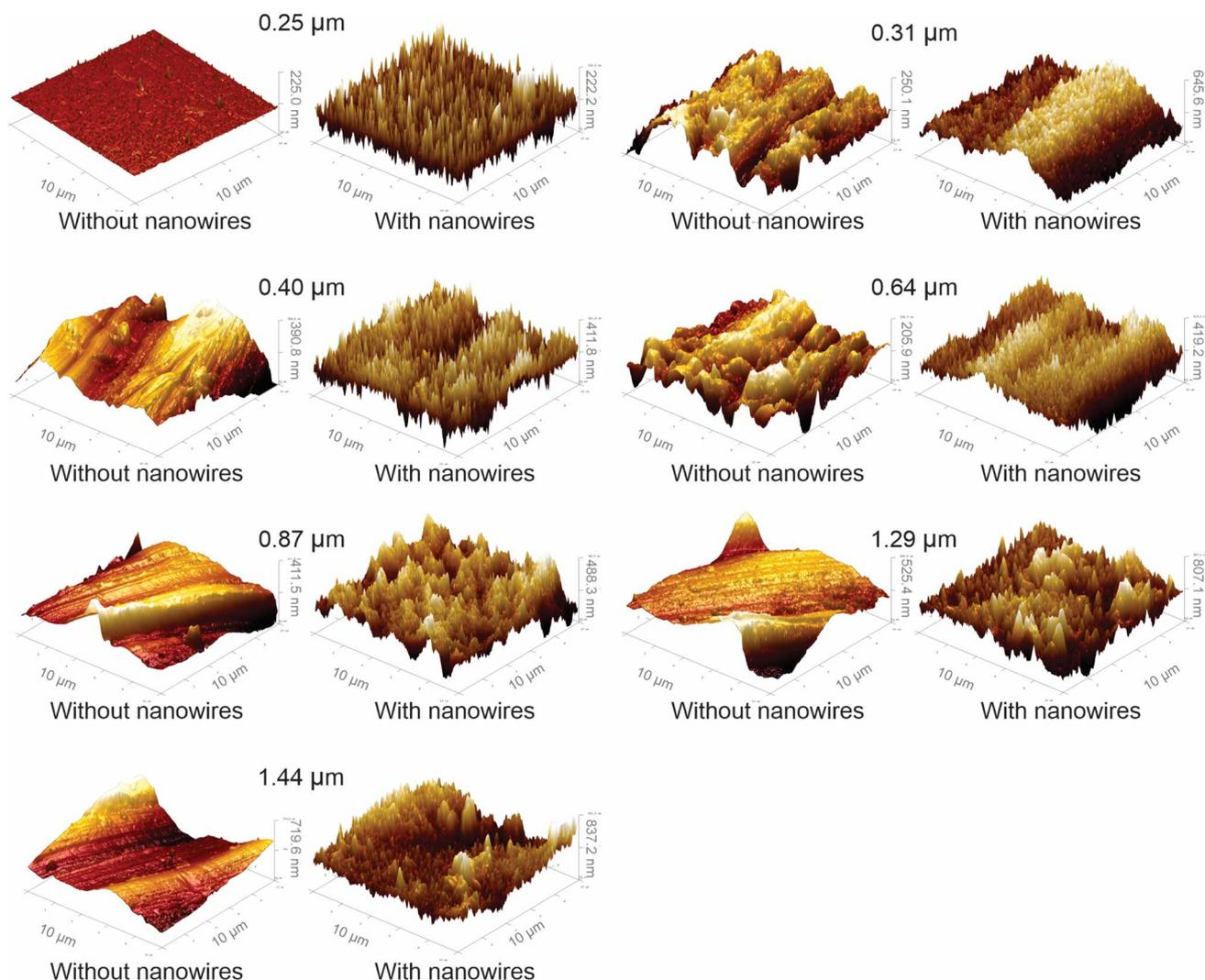
**Fig. 2** Atomic force microscopy images of seven surface groups before and after hydrothermal treatment. Each scan was taken in a  $10\ \mu\text{m} \times 10\ \mu\text{m}$  area on the surface. Atomic force microscopy (AFM). Bruker AFM (Bruker Icon Dimension, Germany) was used with Scanasyt tip in tapping mode. A scan size of  $10\ \mu\text{m}$  with 256 histogram bins and  $0.1\ \text{Hz}$  scan rate was used. 1st order flattening, and 1st order plane fit with  $0.4$  aspect ratio was used.
