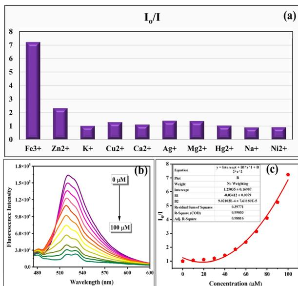
Fig. 2 Relative emission of FHP in the presence of different analytes (100 μM) (a). Fluorescence emission of FHP with increasing Fe<sup>3+</sup> concentrations (0–100 μM) in H<sub>2</sub>O/DMF (4/1, v/v) system (b) and Stern–Volmer plot of FHP against Fe<sup>3+</sup> (0–100 μM) (c).
