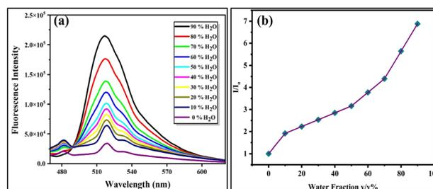
Fig. 1 Emission spectrum of **FHP** with increasing water fraction (0–90%) (a) and relative emission intensity of the probe in increasing water fractions (0–90%) (b).
