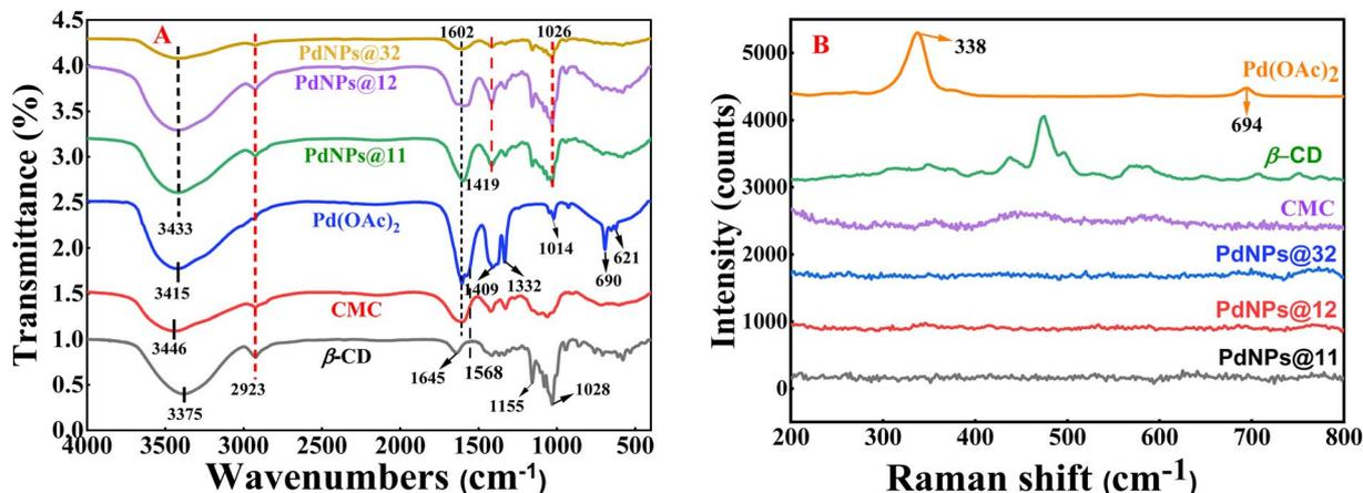
Fig. 5 (A) FT-IR spectra of PdNPs@β-CD-CMC, Pd(OAc)<sub>2</sub>, CMC and β-CD; and (B) Raman spectra of PdNPs@β-CD-CMC, Pd(OAc)<sub>2</sub>, CMC and β-CD.
