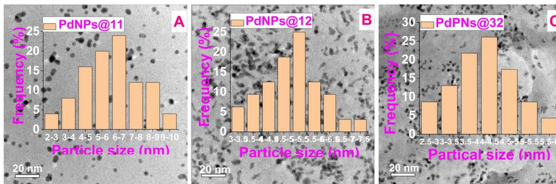
Fig. 7 TEM image of PdNPs@11, PdNPs@12, PdNPs@32.
