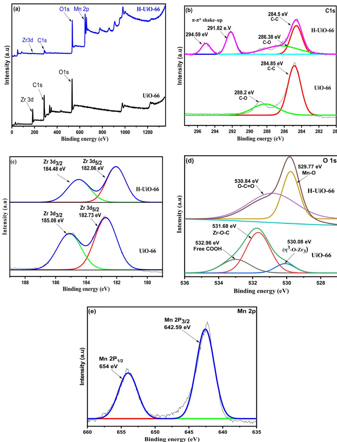
Fig. 5 XPS analysis of UiO-66 and H-UiO-66: (a) survey spectra of elements and XPS spectra high resolution of C 1s (b), Zr 2d (c), O 1s (d), and Mn 2p (e).
