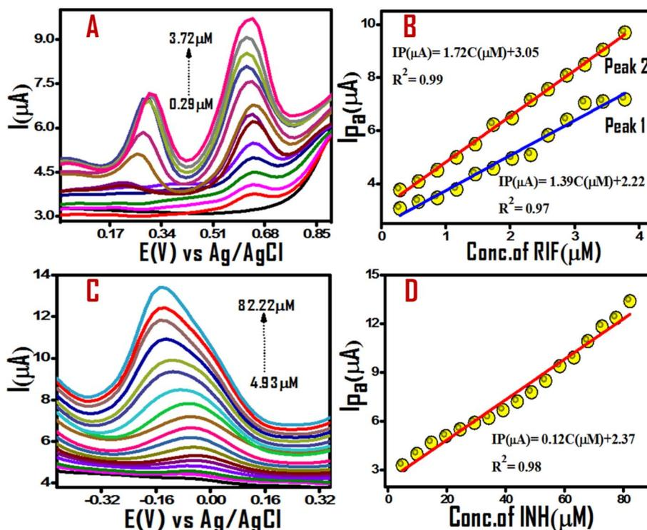
Fig. 6 DPVs recorded for increasing concentrations of (A) RIF and (C) INH on GCE/Ru(II) half sandwich complex. Calibration plots (B and D) between I<sub>p</sub> vs. concentration (μM) of RIF and INH with linear behaviour in concentration range of 0.29–3.72 μM and 4.93–82.22 μM respectively (experiments were attempted in acetonitrile solvent using NBu<sub>4</sub>PF<sub>6</sub> as supporting electrolyte).
