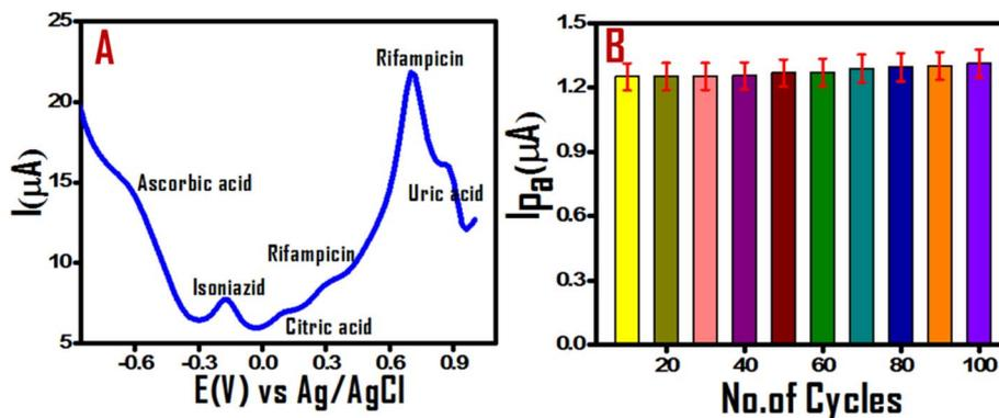
Fig. 9 DPVs recorded on GCE/Ru(II) half sandwich complex (A) for RIF and INH (19.4  $\mu\text{M}$  each) in presence of potential redox active biological interferences (B) stability test of GCE/Ru(II) half sandwich complex. Current measurements were made in aqueous acetonitrile solvent using  $\text{NBu}_4\text{PF}_6$  as supporting electrolyte at scan rate of  $50 \text{ mV s}^{-1}$  in case of (A) and  $100 \text{ mV s}^{-1}$  in case of (B).
