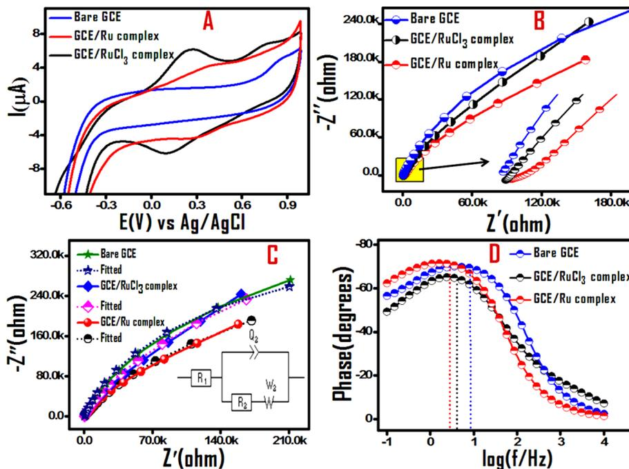
Fig. 2 (A) Comparative cyclic voltammograms recorded at scan rate of  $100 \text{ mV s}^{-1}$  of bare GCE, GCE/Ru(II) half sandwich complex and GCE/RuCl<sub>3</sub>, (B and C) Nyquist plots and equivalent circuit model for fitting EIS data, and (D) Bode phase plots of bare GCE, GCE/Ru salt and GCE/Ru(II) half sandwich complex obtained at a frequency range of 10 kHz to 100 mHz (all experiments were performed in acetonitrile solvent using NBu<sub>4</sub>PF<sub>6</sub> as supporting electrolyte).
