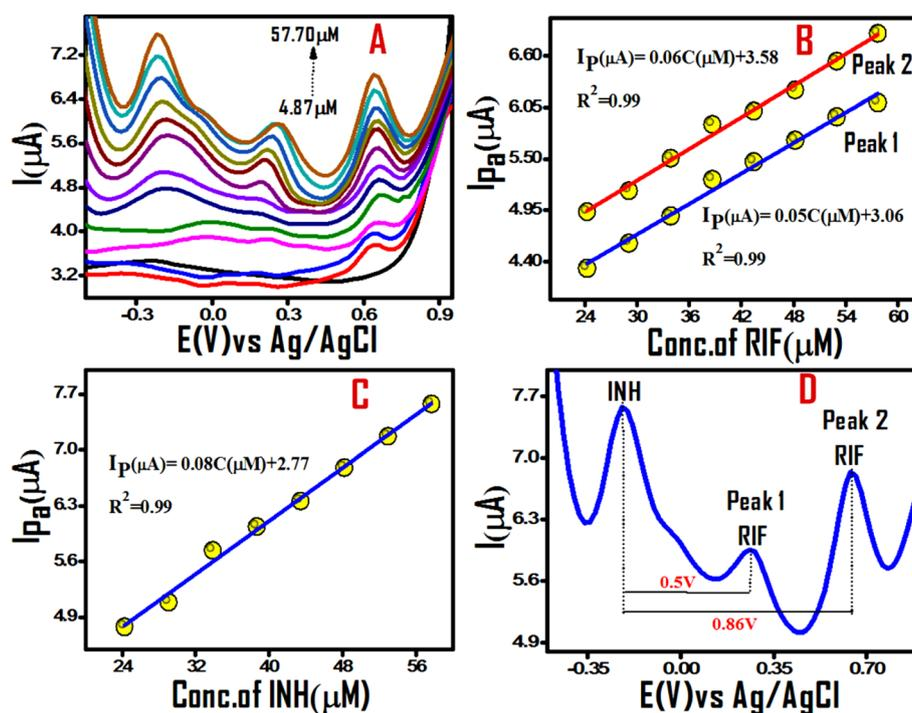
Fig. 8 DPVs recorded on GCE/Ru(II) half sandwich complex (A) for simultaneous determination of increasing concentrations 4.87–57.69  $\mu\text{M}$  of RIF and INH. Calibration plots of the peak current against concentration of analytes (B and C). Plot showing separations between the peak potentials of RIF and INH (D). (All measurements were in acetonitrile solvent using  $\text{NBu}_4\text{PF}_6$  as supporting electrolyte at scan rate of  $50 \text{ mV s}^{-1}$ ).
