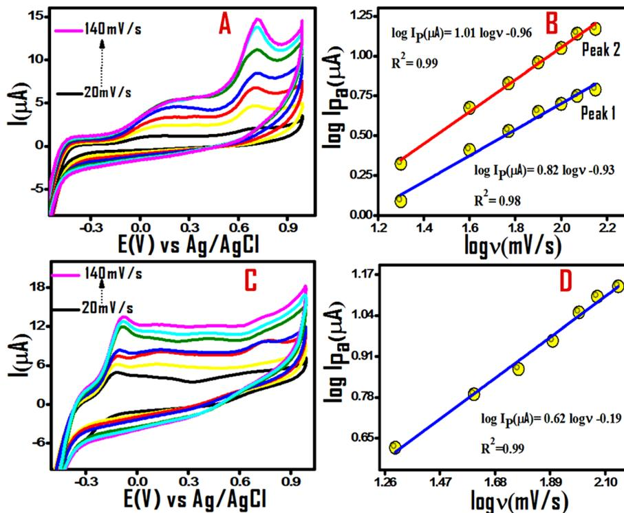
Fig. 5 Cyclic voltammograms recorded on GCE/Ru(II) half sandwich complex with changing scan rates (20–140 mV s<sup>-1</sup>) (A) 5.4 μM RIF (C) 138 μM INH (B and D) linear fit plots between log I<sub>p</sub> vs. log ν obtained for anodic peak currents of RIF and INH respectively (CV experiments were performed in aqueous acetonitrile solvent with NBu<sub>4</sub>PF<sub>6</sub> as supporting electrolyte).
