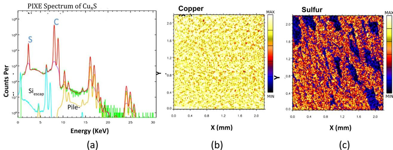
Fig. 3 PIXE analysis of  $\text{Cu}_2\text{S}$  nanostructures. (a) PIXE spectrum showing characteristic X-ray emission peaks for copper ( $\text{Cu K}\alpha$ ) and sulfur ( $\text{S K}\alpha$ ). (b) Elemental mapping of copper (Cu), illustrating uniform spatial distribution across the nanostructure surface. (c) Elemental mapping of sulfur (S), confirming homogeneous distribution consistent with the copper distribution.
