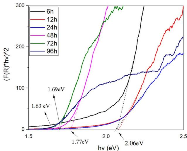
Fig. 5 Band gap energy estimation of  $\text{Cu}_2\text{S}$  samples synthesized at different exposure times (6 h, 12 h, 24 h, 48 h, 72 h, 96 h) using the Kubelka–Munk function. The plots of  $(F(R) \times hv)^2$  vs. photon energy ( $h\nu$ ) show a decrease in band gap from 2.06 eV (6 h) to 1.63 eV (96 h), indicating changes in the material's electronic structure with extended synthesis.
