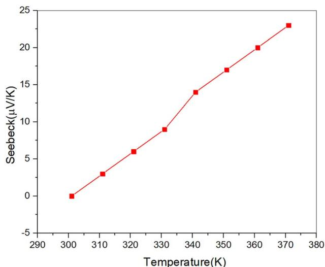
Fig. 9 Temperature-dependent Seebeck coefficient of the 96 h Cu<sub>2</sub>S sample. The positive Seebeck values across all temperatures confirm p-type behavior, with a peak value of approximately 20 μV K<sup>-1</sup> at higher temperatures. Variations in the coefficient suggest the influence of polymorphic transitions, indicating the material's potential for thermoelectric applications.
