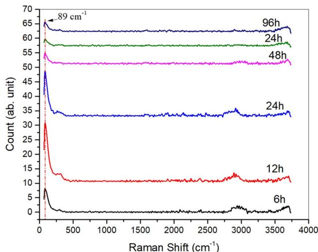
Fig. 6 Raman spectra of  $\text{Cu}_2\text{S}$  samples synthesized at varying exposure times (6 h, 12 h, 24 h, 48 h, 72 h, 96 h). The absence of characteristic  $\text{Cu}_2\text{S}$  peaks indicates an amorphous phase, while observed  $\text{Cu}_2\text{O}$  peaks suggest surface oxidation, likely affecting the material's optical and electrical properties.
