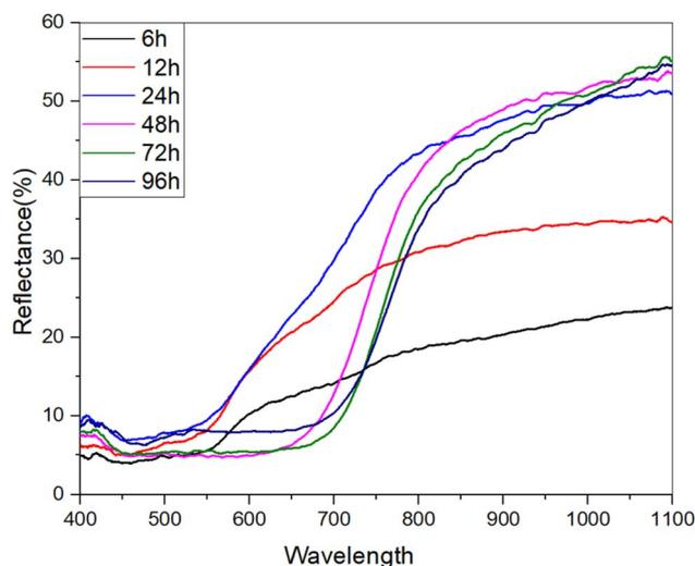
Fig. 4 Diffuse reflectance spectroscopy (DRS) spectra of  $\text{Cu}_2\text{S}$  samples synthesized at different exposure times (6 h, 12 h, 24 h, 48 h, 72 h, 96 h) over 400–1100 nm. Low reflectance within the visible range (400–600 nm) indicates effective light absorption, while a sharp increase beyond 700 nm suggests a shift towards the near-infrared region. The rise between 600 and 700 nm marks the absorption threshold, reflecting the time-dependent evolution of optical properties.
