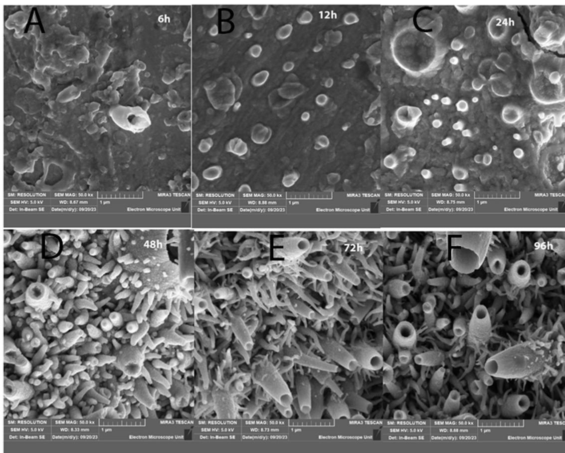
Fig. 1 Surface morphology of Cu substrate exposed to garlic-derived organosulfur compounds for varying durations observed *via* FESEM at 1  $\mu\text{m}$  resolution. Images depict samples after (a) 6 h, (b) 12 h, (c) 24 h, (d) 48 h, (e) 72 h, and (f) 96 h exposure times. Prolonged exposure (48 h, 72 h, and 96 h) leads to pronounced nanostructure formation, resembling tubular sea coral reefs, indicating the progressive impact of time-dependent sulfurization on nanostructure development.
