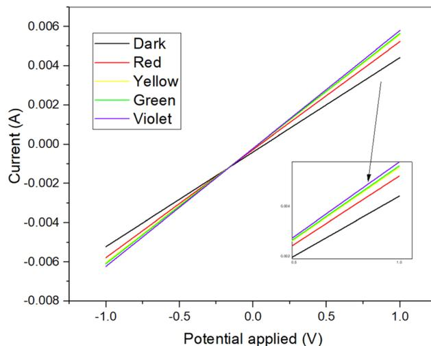
Fig. 7 Current–voltage ( $I$ – $V$ ) characteristics of the 96 h  $\text{Cu}_2\text{S}$  sample measured in the dark and under illumination with different wavelengths (red, yellow, green, violet). The linear curves indicate consistent ohmic behavior, with slight variations in resistance under light exposure. The increased current response with shorter wavelengths demonstrates the material's sensitivity to higher-energy light, suggesting potential for optoelectronic applications.
