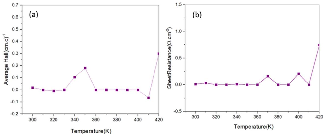
Fig. 8 Temperature-dependent electrical properties of the 96 h Cu<sub>2</sub>S sample. (a) Hall coefficient measurements confirm p-type conductivity, indicating holes as the dominant charge carriers. (b) Sheet resistance increases slightly at 420 K, reflecting typical semiconductor behavior where higher temperatures lead to increased carrier scattering and reduced mobility. These insights are crucial for assessing the material's thermoelectric potential.
