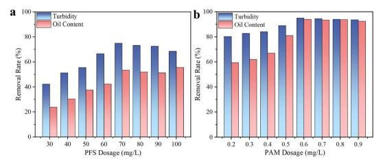
Fig. 10 Pollutant removal efficiency of the MCFR under different reagent addition amounts. (a) PFS addition amount, (b) PAM addition amount (operate at a flow rate of  $100 L h^{-1}$ , a setting time of 30 minutes, and 20 °C).
