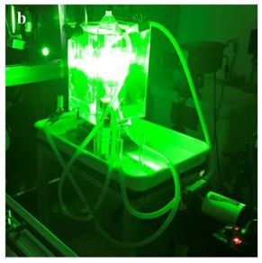
Fig. 2 Actual images of PIV shooting. (a) Before shooting: (1) laser transmitter, (2) MCFR, (3) CCD camera, (4) power pump, (b) shooting process.
