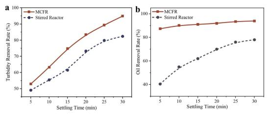
Fig. 12 Comparison of pollutant removal efficiency between the MCFR and a stirred reactor at different settling times. (a) Turbidity removal rate, (b) oil content removal rate (operate at PFS and PAM dosages of 70 mg  $L^{-1}$  and 0.6 mg  $L^{-1}$ , and 20 °C, MCFR operate at a flow rate of 100 L  $h^{-1}$ ).
