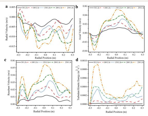
Velocity and energy distribution curves of section B. (a) Radial velocity, (b) axial velocity, (c) resultant velocity, (d) turbulent kinetic energy.
