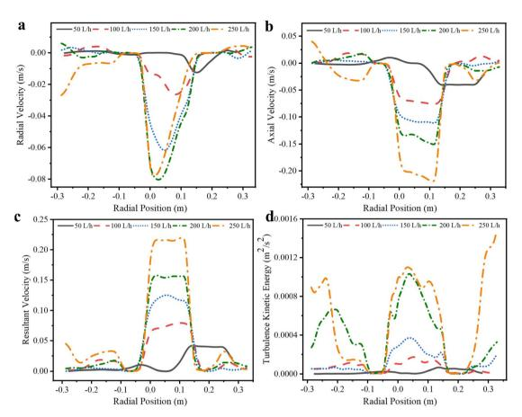
Fig. 9 Velocity and energy distribution curves of section E. (a) Radial velocity, (b) axial velocity, (c) resultant velocity, (d) turbulent kinetic energy.
