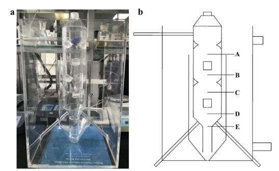
Physical picture (a) and characteristic cross-section diagram (b) of the MCFR.
