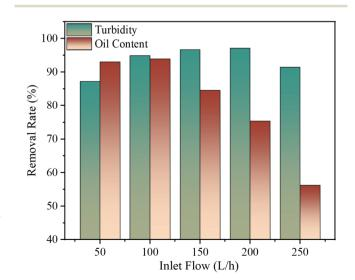
Fig. 11 Pollutant removal efficiency of the MCFR at different inlet flow rates (operate at PFS and PAM dosages of 70 mg  $L^{-1}$  and 0.6 mg  $L^{-1}$ , a setting time of 30 minutes, and 20 °C).
