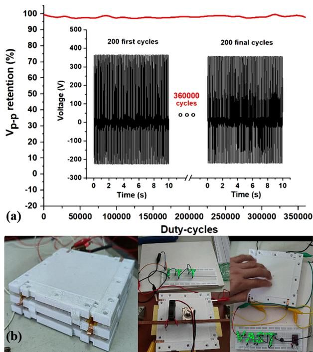
Fig. 6 Output voltage decline of a 3D printed PHMG-GA-PVA TENG device after 360 000 working cycles (a) and photos of a TENG module used to power for LEDs (b).
