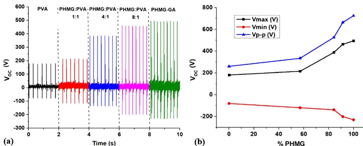
Fig. 4 (a) Open circuit voltages ( $V_{OC}$ ) of PVA, PHMG-GA-PVA and PHMG-GA electrodes prepared at different ratios of PHMG-GA/PVA; (b) maximum ( $V_{max}$ ), minimum ( $V_{min}$ ), and peak-to-peak ( $V_{p-p}$ ) voltages of  $V_{OC}$  as a function of PHMG content.
