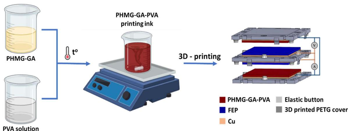
Fig. 1 Illustration of the fabrication process for PHMG-GA-PVA TENG electrodes.
