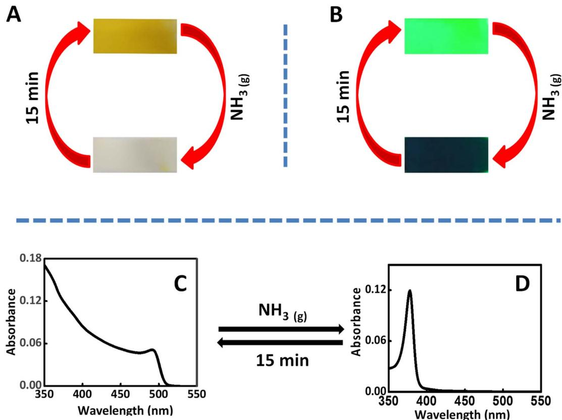
Fig. 2 The influence of ammonia intercalation on the properties of CsPbBr<sub>3</sub> perovskite Nanocrystals. (A) Photographs showing the reversible intercalation of ammonia vapors in the CsPbBr<sub>3</sub> crystals coated on a paper substrate viewed under normal light and (B) ultraviolet light. UV-visible absorption spectra of CsPbBr<sub>3</sub> nanocrystals before (C) and after (D) ammonia intercalation.
