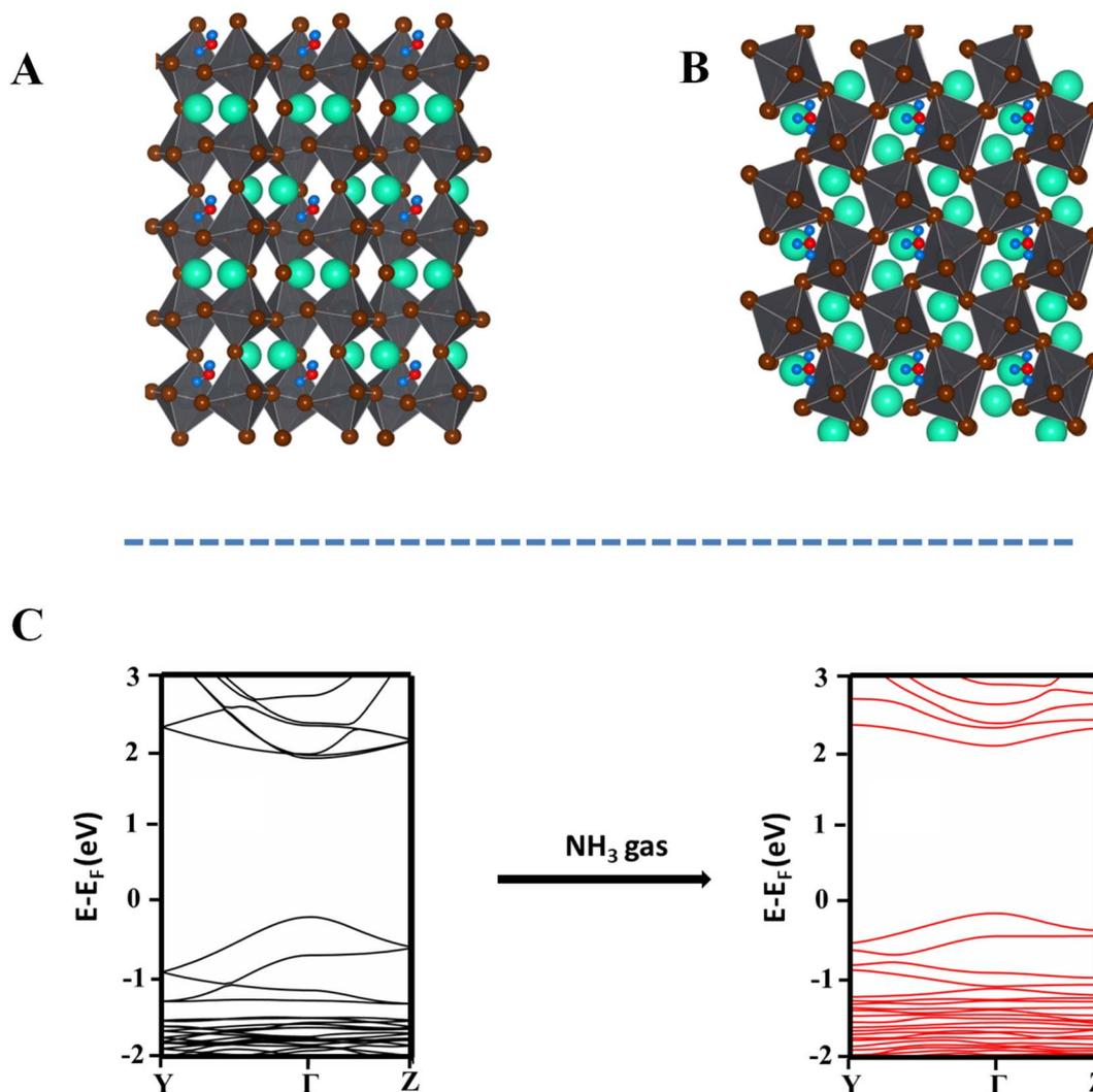
Fig. 3 The optimized geometry of  $\text{NH}_3$  intercalated  $\text{CsPbBr}_3$  perovskite (A) side view and (B) top view. The band structure plot for (C) pristine  $\text{CsPbBr}_3$  before and after intercalation of ammonia.
