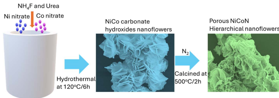
Fig. 1 Schematic of synthesis hierarchical NiCoN porous nanoflower-sheets.
