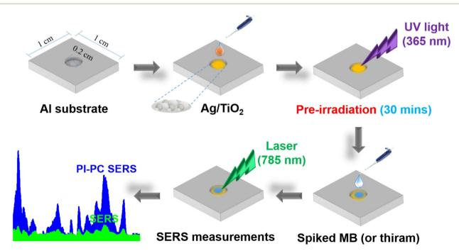
Scheme 1 Pre-irradiation procedure of Ag/TiO<sub>2</sub> SERS substrate in the PI-PC SERS technique for enhancing the SERS signal via the PIERS effect.
