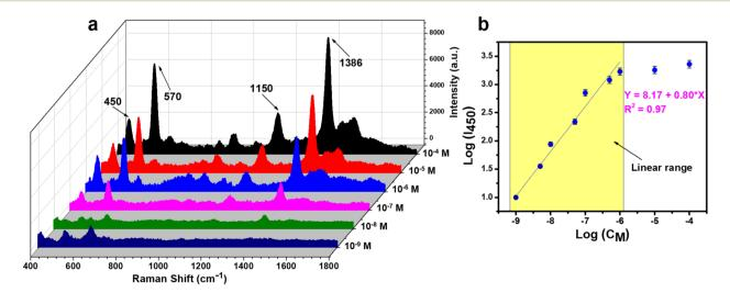
Fig. 5 SERS spectra of thiram in the concentration range of  $10^{-4}$  to  $10^{-9}$  M under normal SERS conditions (a), and the linear relationship between thiram concentration and SERS intensity on a logarithmic scale (b).
