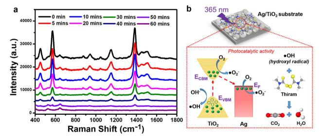
Fig. 8 Photocatalytic activity of the Ag/TiO<sub>2</sub> SERS substrate in thiram degradation monitored by SERS spectra (a), and the mechanism of thiram degradation by the Ag/TiO<sub>2</sub> nanostructure under UV 365 nm irradiation (b).
