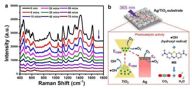
Fig. 4 Photocatalytic activity of the  $Ag/TiO_2$  SERS substrate in MB degradation monitored by SERS spectra (a), and the mechanism of MB degradation by the  $Ag/TiO_2$  nanostructure under UV 365 nm irradiation (b).
