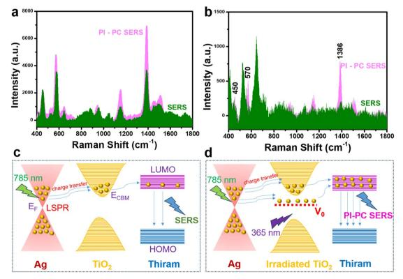
Fig. 7 Comparison of SERS intensity of thiram between normal SERS and PI-PC SERS techniques at concentrations of  $10^{-6}$  M (a) and  $10^{-9}$  M (b). Mechanism of normal SERS of the Ag/TiO<sub>2</sub> substrate in thiram detection (c) and mechanism of enhanced SERS signal in PI-PC SERS of the Ag/TiO<sub>2</sub> substrate (d).
