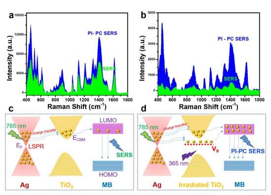
Fig. 3 Comparison of SERS intensity of MB between normal SERS and PI-PC SERS techniques at concentrations of  $10^{-6}$  M (a) and  $10^{-10}$  M (b). Mechanism of normal SERS of the Ag/TiO<sub>2</sub> substrate in MB detection (c) and mechanism of enhanced SERS signal in PI-PC SERS of the Ag/TiO<sub>2</sub> substrate (d).
