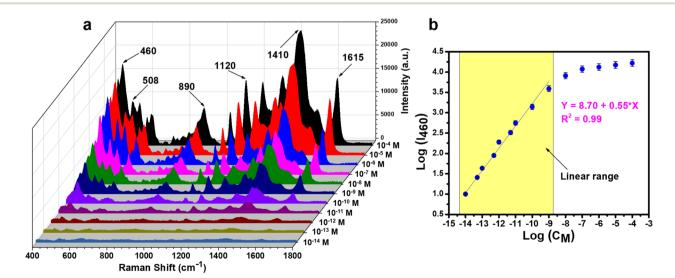
Fig. 2 SERS spectra of MB in the concentration range of  $10^{-4}$  to  $10^{-14}$  M under PI-PC SERS technique (a), and the linear relationship between MB concentration and SERS intensity on a logarithmic scale (b).
