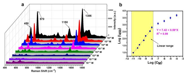
Fig. 6 SERS spectra of thiram in the concentration range of  $10^{-4}$  to  $10^{-11}$  M under PI-PC SERS technique (a), and the linear relationship between thiram concentration and SERS intensity on a logarithmic scale (b).
