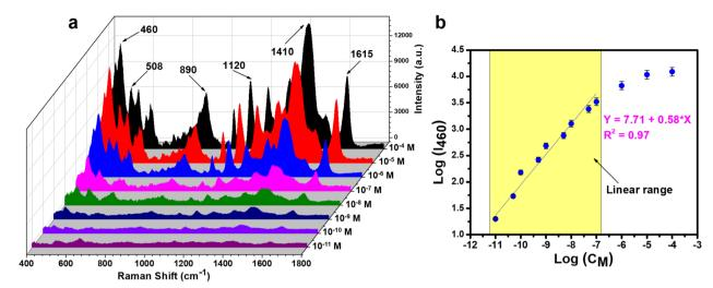
Fig. 1 SERS spectra of MB in the concentration range of  $10^{-4}$  M to  $10^{-11}$  M under normal SERS conditions (a), and the linear relationship between MB concentration and SERS intensity on a logarithmic scale (b).
