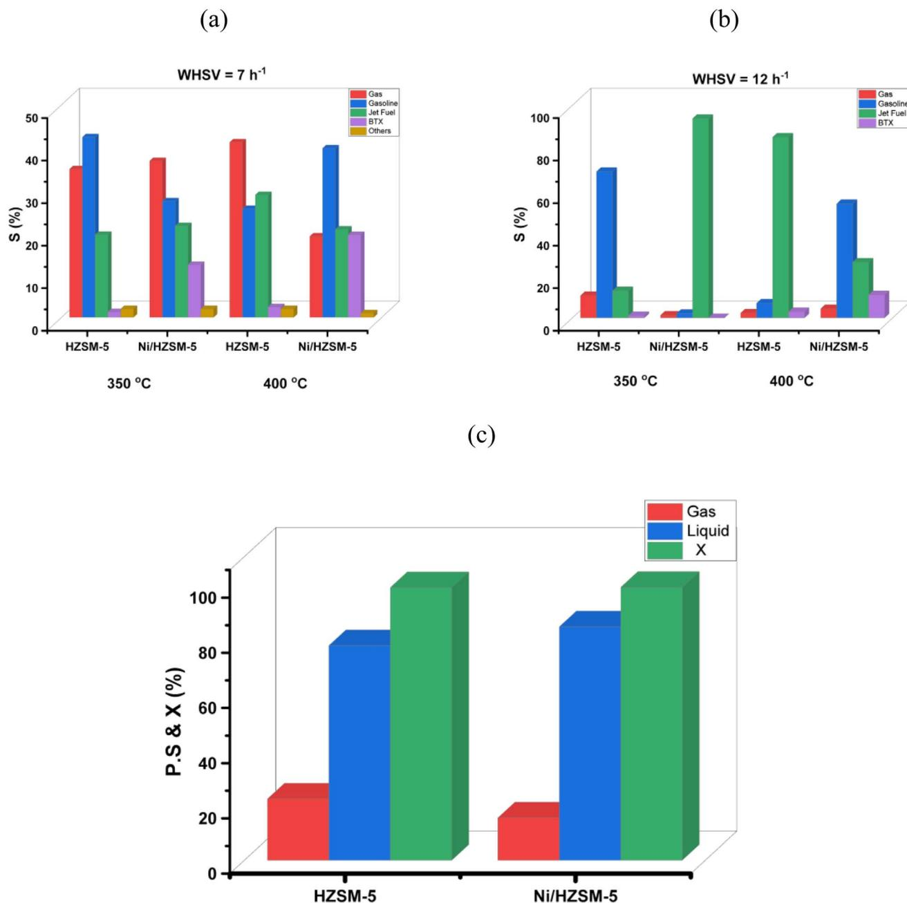
Fig. 1 Product selectivity (S) over HZSM-5 and Ni/HZSM-5 at (a) 7 h<sup>-1</sup> and (b) 12 h<sup>-1</sup> WHSV (c) average phase selectivity (P.S) and conversion (X) from the 1-propanol conversion to fuel blendstock. Reaction conditions: 350 and 400 °C; WHSV = 7 and 12 h<sup>-1</sup>.
