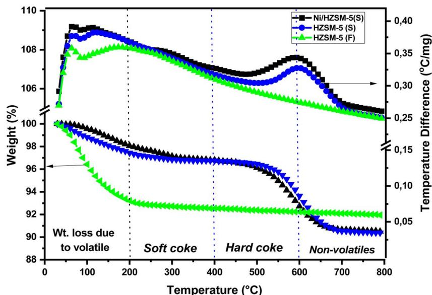
Fig. 7 TGA-DTA of spent HZSM-5 and Ni/HZSM-5 catalysts.
