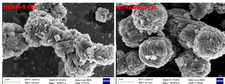
Fig. 5 SEM of spent HZSM-5 and Ni/HZSM-5 catalysts.
