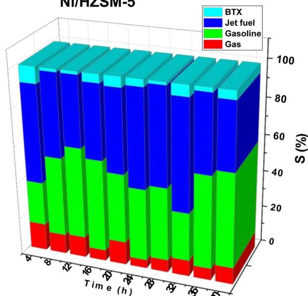
Fig. 3 Catalyst stability study at  $7\text{ h}^{-1}$  and  $350\text{ }^\circ\text{C}$  for 40 h TOS showing (a) 1-propanol conversion (X), and product distribution for (b) HZSM-5 (c) Ni/HZSM-5 catalysts.
