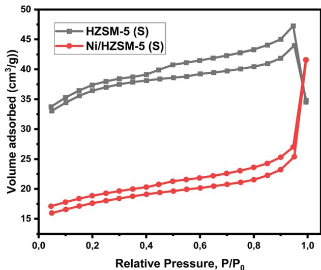
Fig. 6  $N_2$  adsorption-desorption isotherm for spent catalysts.
