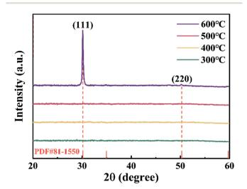
Fig. 3 XRD pattern of  ${\rm ZrGdO}_{\rm X}$  thin films at different annealing temperatures.
