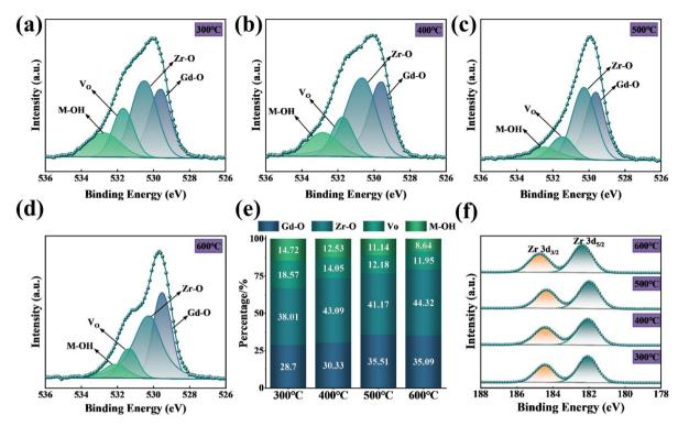
Fig. 5 O 1s spectra of ZrGdO<sub>x</sub> films annealed at (a) 300 °C, (b) 400 °C, (c) 500 °C, (d) 600 °C, (e) atomic percentages of the oxygen components in each sample, (f) XPS spectra of Zr 3d
