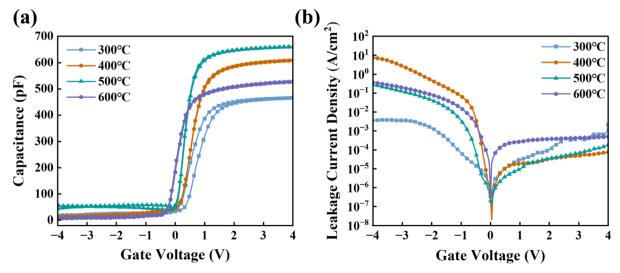
Fig. 9 (a) C-V and (b) J-V curves of the MOS capacitors based on ZrGdO<sub>v</sub> films.
