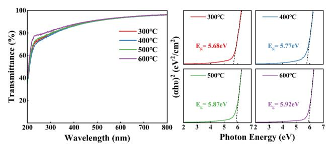
Fig. 6 (a) Transmittance and (b) optical band gaps spectra of ZrGdO<sub>x</sub> thin films at various annealing temperatures.
