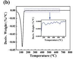
Fig. 2 (a) TG and (b) DTG curves of ZrGdO<sub>x</sub> precursor.
