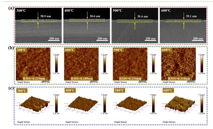
Fig. 8 (a) Cross-sectional SEM patterns of ZrGdO<sub>x</sub> thin films, (b) 2D and (c) 3D AFM maps of the samples at different annealing temperatures, respectively.
