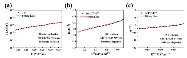
Fig. 10 (a) Ohmic conduction, (b) SE emission, and (c) P-F emission plots of Al/ZrGdO<sub>x</sub>/Si capacitors in substrate injection mode.
