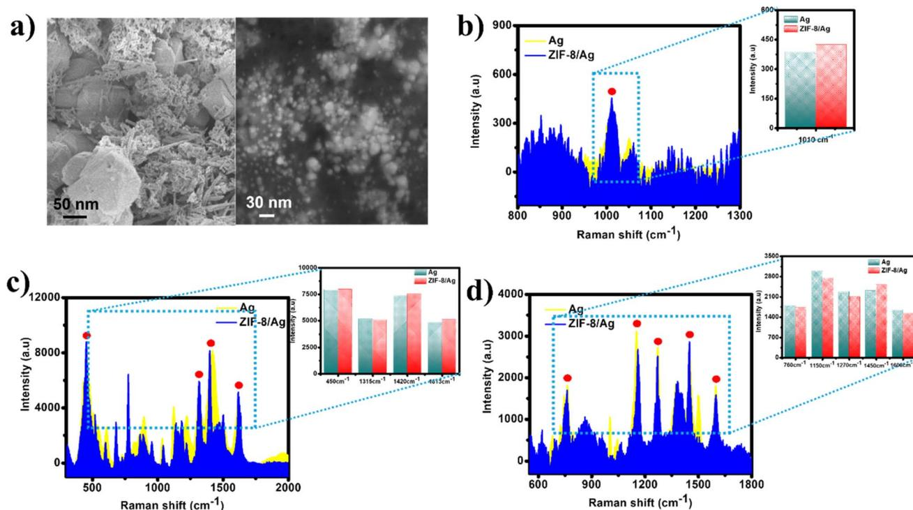
Fig. 6 (a) SEM image of ZIF-8 (left) and ZIF-8/Ag (right) treated with ultrasonication; SERS intensities at characteristic peaks of (b) urea ( $10^{-3}$  M), (c), MB ( $10^{-5}$  M), and (d) CR ( $10^{-4}$  M) on AgNPs and ZIP-8/Ag, in which ZIP-8 frames was destroyed after ultrasonication treatment.
