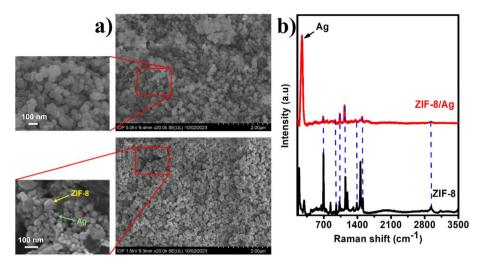
Fig. 1 (a) and (b) SEM images of ZIF and ZIF/Ag, respectively; (b) Raman spectra of ZIF-8 and ZIF-8/Ag.
