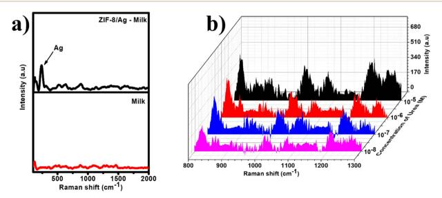
Fig. 9 (a) Raman spectrum of milk (red) and SERS spectrum of milk on ZIF-8/Ag (black); (b) SERS spectra of urea at different concentrations in real samples of milk on ZIF-8/Ag substrates.
