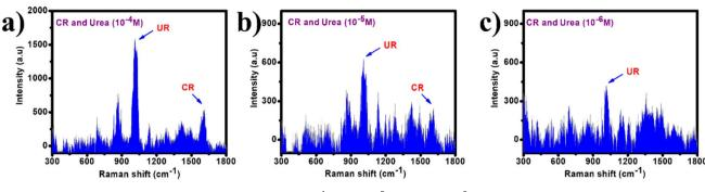
Fig. 8 SERS spectra of solutions containing urea and CR (a)  $10^{-4}$  M, (b)  $10^{-5}$  M, and (c)  $10^{-6}$  M on ZIF-8/Ag.
