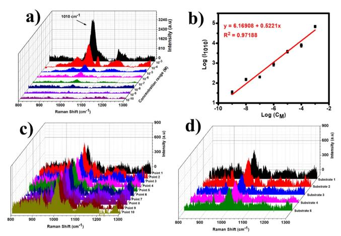
Fig. 7 (a) SERS spectra of urea  $(10^{-3} \text{ M to } 10^{-10} \text{ M})$  on ZIF-8/Ag. (b) The plot of the log of SERS intensity at 1010 cm<sup>-1</sup> against urea concentration. (c) Uniformity and (d) reproducibility of SERS sensors for urea on ZIF-8/Ag substrate.
