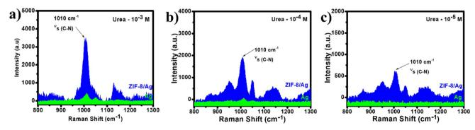
Fig. 2 SERS spectra of urea at  $10^{-3}$  M (a),  $10^{-4}$  M (b) and  $10^{-5}$  M (c) on AqNPs and ZIP-8/Aq substrates.
