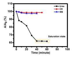
Fig. 5 Changes in relative concentration of urea, MB and CR in the presence of ZIF-8/Ag in solution during incubation time.
