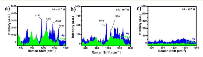
Fig. 4 SERS spectra of CR at  $10^{-4}$  M (a),  $10^{-5}$  M (b) and  $10^{-6}$  M (c) on AqNPs and ZIP-8/Aq substrates.
