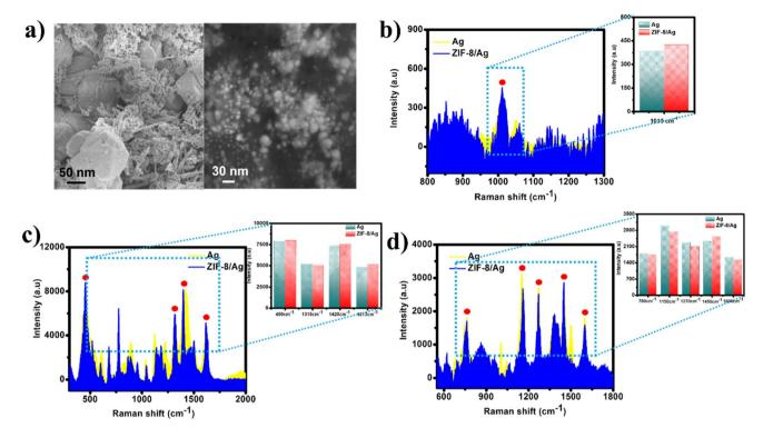
Fig. 6 (a) SEM image of ZIF-8 (left) and ZIF-8/Ag (right) treated with ultrasonication; SERS intensities at characteristic peaks of (b) urea (10<sup>-3</sup> M), (c), MB (10<sup>-5</sup> M), and (d) CR (10<sup>-4</sup> M) on AgNPs and ZIP-8/Ag, in which ZIP-8 frames was destroyed after ultrasonication treatment.
