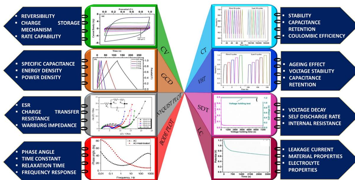
Fig. 16 Schematic of the roles of BDAC material in an electrochemical system.
