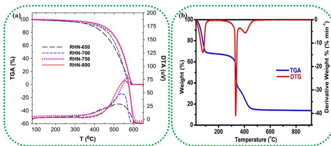
Fig. 2 (a) TGA/DTA analysis of pinewood-derived activated carbon using different activating agents, such as H<sub>3</sub>PO<sub>4</sub>, KOH, and H<sub>2</sub>O<sub>2</sub>, and heat-only treatments. Reprinted with permission from ref. 93, copyright 2014, Elsevier. (b) TGA/DTG analysis of activated carbon prepared from rice husk at 850 °C under an O<sub>2</sub> atmosphere. Reprinted with permission from ref. 94, copyright 2016, Elsevier.
