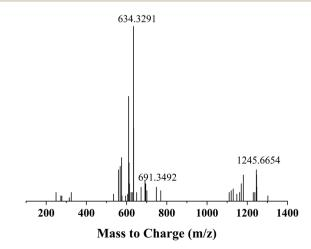
Fig. 4 The high resolution mass spectrum of GBSilane.
