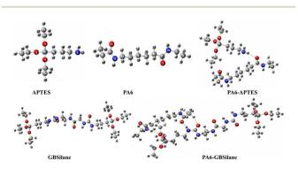
Fig. 8 Optimized molecular configuration of APTES, PA6 and GBSilane, along with hydrogen bonds information between PA6-APTES and PA6-GBSilane.
