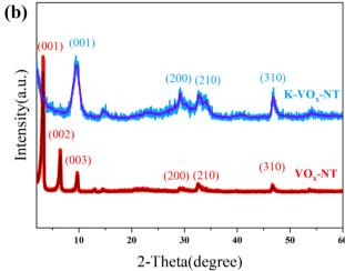
Fig. 1 (a) Schematic of the microstructure of  $VO_x$ -NT and illustration of the K<sup>+</sup> exchange process; (b) XRD patterns and relevant fittings of  $VO_x$ -NT and K- $VO_x$ -NT.
