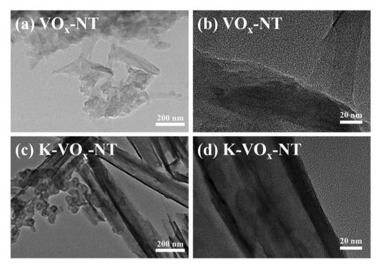
Fig. 7 TEM images of  $VO_x$ -NT (a, b) and K-VO<sub>x</sub>-NT (c, d) at different magnifications after 100 cycles.
