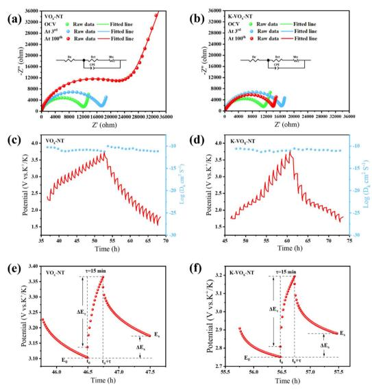
Fig. 8 Nyquist plots of VO<sub>x</sub>-NT (a) and K-VO<sub>x</sub>-NT (b) from EIS tests at OCV and the 1st and 100th cycles; potential response curves during GITT measurements and the corresponding logarithm of K<sup>+</sup> diffusion coefficients ( $D_{K^+}$ ) for VO<sub>x</sub>-NT (c) and K-VO<sub>x</sub>-NT (d); representative processes (e and f) of single pulse and relaxation during GITT measurements for the two samples.
