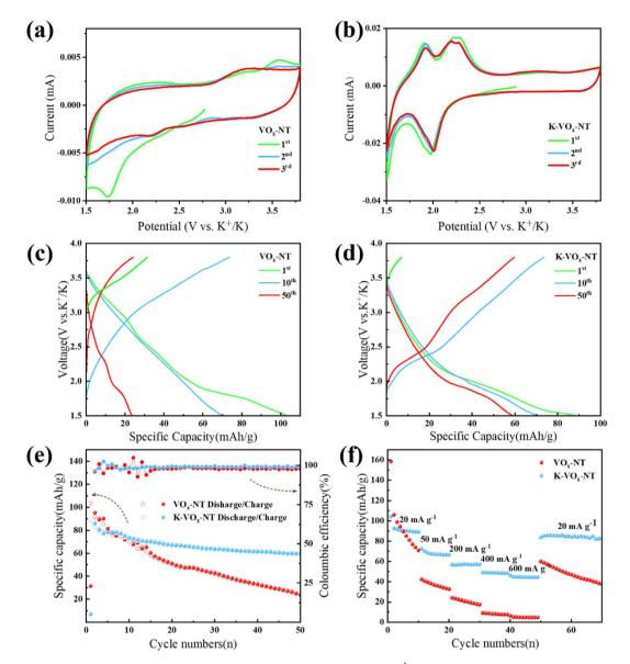
Fig. 6 Initial three CV curves of  $VO_x$ -NT (a) and K- $VO_x$ -NT (b) at a scan rate of 0.2 mV s<sup>-1</sup>; GCD profiles at the 1st, 10th and 50th cycles for  $VO_x$ -NT (c) and K-VO<sub>x</sub>-NT (d) under 50 mA  $g^{-1}$  in the voltage region of 1.5–3.8 V; cycling performances (e) under 50 mA  $g^{-1}$  and rate capabilities (f) for VO<sub>x</sub>-NT and K-VO<sub>x</sub>-NT under different current densities
