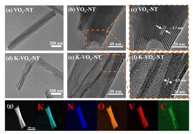
Fig. 2 TEM and HR-TEM images of VO<sub>x</sub>-NT (a-c) and K-VO<sub>x</sub>-NT (d-f); HAADF image and the corresponding elemental mappings for K-VO<sub>x</sub>-NT (a).
