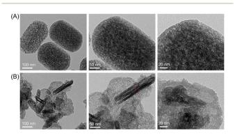
Fig. 3 (A) TEM image of  $SiO_2$  nanoparticles, (B) TEM image of 5MgMSNs. The red arrows indicate the thickness of 5MgMSNs.
