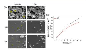
Fig. 6 (A) Biodegradation behavior of 5MgMSNs and SiO<sub>2</sub>. Highlighted in yellow are select nanosheets, indicating their transformation preand post-degradation. (B) Accumulated releasing profiles of Mg ions.
