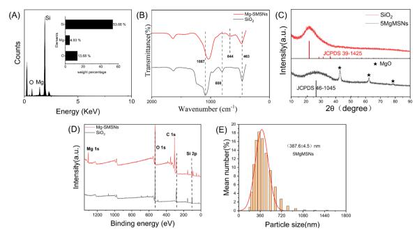
Fig. 2 (A) EDS spectrum of SMGMSNs, (B) FT-IR spectra of  $SiO_2$  and SMGMSNs, (C) XRD pattern of  $SiO_2$  and SMGMSNs, (D) XPS spectrum of  $SiO_2$  and SMGMSNs, (E) size distribution of the SMGMSNs.
