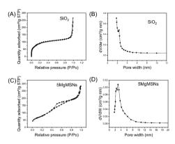
Fig. 4 (A) N<sub>2</sub> adsorption-desorption isotherm and (B) corresponding pore-size distribution of SiO<sub>2</sub>. (C) N<sub>2</sub> adsorption-desorption isotherm and (D) corresponding pore-size distribution of 5MgMSNs.
