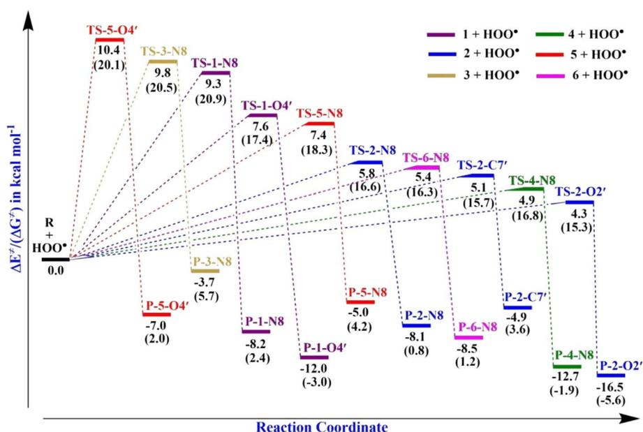
Fig. 4 PES for the reactions of the hydrazone compounds with HOO<sup>•</sup> in the gas phase.
