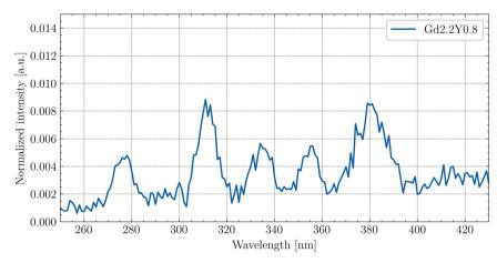
Fig. 12 Enlarged RL spectrum of Gd<sub>2.2</sub>Y<sub>0.8</sub> at RT in the 250–430 nm range.
