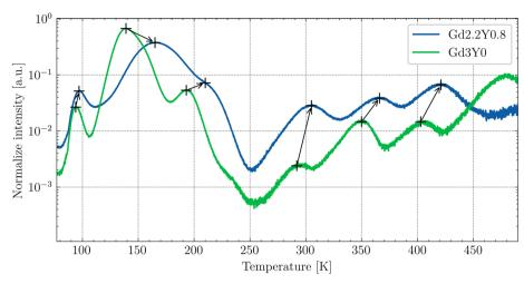
Fig. 10 TSL glow curves for the temperature range of 77-500 K for  $Gd_{2.2}Y_{0.8}$  and  $Gd_3Y_0$  after irradiation with an X-ray source of 40 kV at 77 K. The peaks are shifted to the higher temperatures with Y-substitution.
