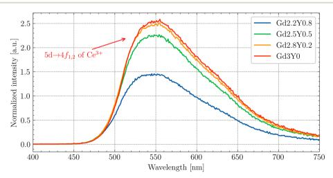
Fig. 11 Radioluminescence spectra of the GYSAG:Ce set. The dominant peak corresponds to the  $Ce^{3+}$  5d<sub>1</sub>-4f<sub>1,2</sub> transition.
