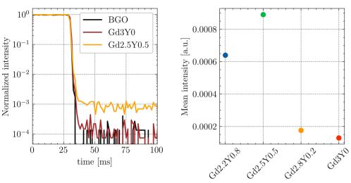
Fig. 14 (A) Normalized afterglow curves of  $Gd_3Y_0$  and  $Gd_{2.5}Y_{0.5}$  samples. (B) Mean afterglow value calculated as a mean of intensities in the range of 20 ms after X-ray cut-off.
