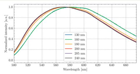
Fig. 7 Dependence of the peak position of Ce<sup>3+</sup> emission on the excitation wavelength at RT for Gd<sub>2.8</sub>Y<sub>0.2</sub>.
