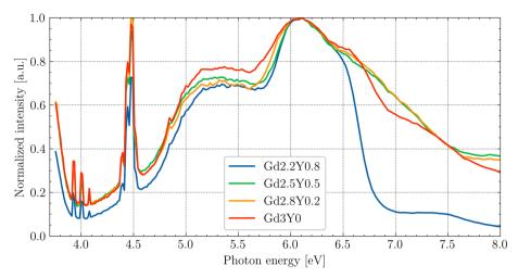
Fig. 6 PLE of  $Ce^{3+}$  (em = 530) under synchrotron radiation at RT. The data are normalized to the excitonic band (6.7 eV).
