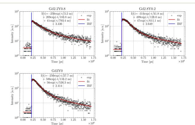
$\textbf{Fig. 13} \quad \text{Scintillation rise time and decay measurement of } Gd_{2.2}Y_{0.8}, Gd_{2.8}Y_{0.2} \text{ and } Gd_{3}Y_{0} \text{ with their fits. Excitation by a picosecond laser-driven X-1} \\$ ray source (40 keV, 75 ps pulse FWHM).
