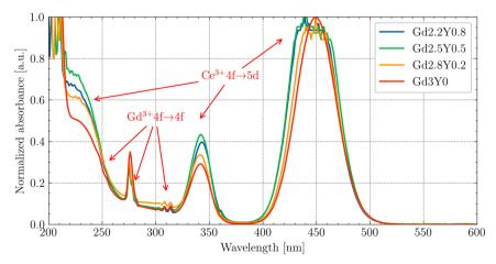
Fig. 3 Absorption spectra of the  $Gd_{2.2}Y_{0.8}$ ,  $Gd_{2.5}Y_{0.5}$ ,  $Gd_{2.8}Y_{0.2}$ ,  $Gd_3Y_0$  samples at RT.
