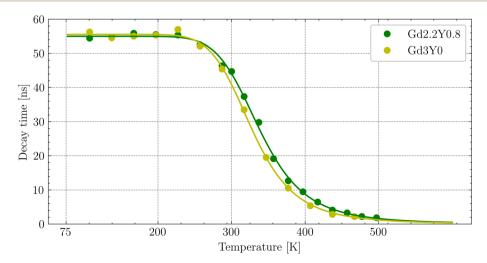
Fig. 9 Temperature dependence of the photoluminescence decay time of  $Ce^{3+}$  (first component of the two-exponential fit) fitted by the curve (green and yellow lines) calculated using the single-barrier quenching model.
