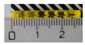
Fig. 1 Photograph of the Gd<sub>2.2</sub>Y<sub>0.8</sub> crystal annealed at 1200 °C for 12 hours (See F in the ESI data† for photographs of other crystals).
