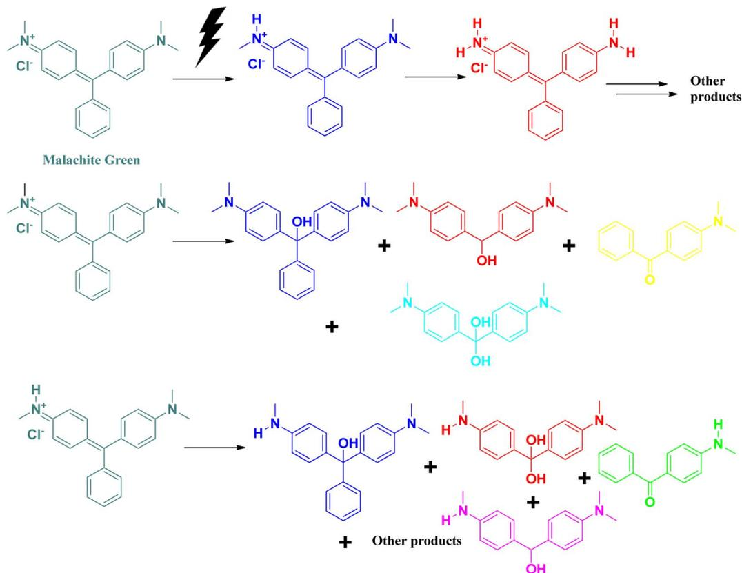
Fig. 11 Probable products of malachite green after photodegradation.
