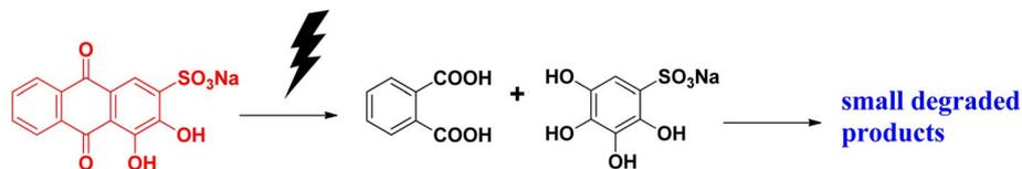
Fig. 10 Photocatalytic degradation of alizarin red S.
